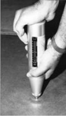
FIGURE 7.34 Rebound hammer for nondestructive evaluation of hardened concrete.
