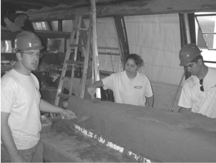
FIGURE 7.43 ASCE students at Arizona State University making a concrete canoe using lightweight concrete.
