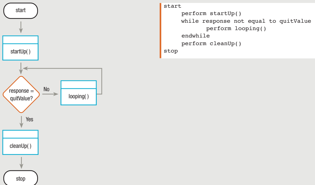
FIGURE 10-19: FLOWCHART AND PSEUDOCODE FOR MAINLINE LOGIC FOR MULTILEVEL MENU PROGRAM
