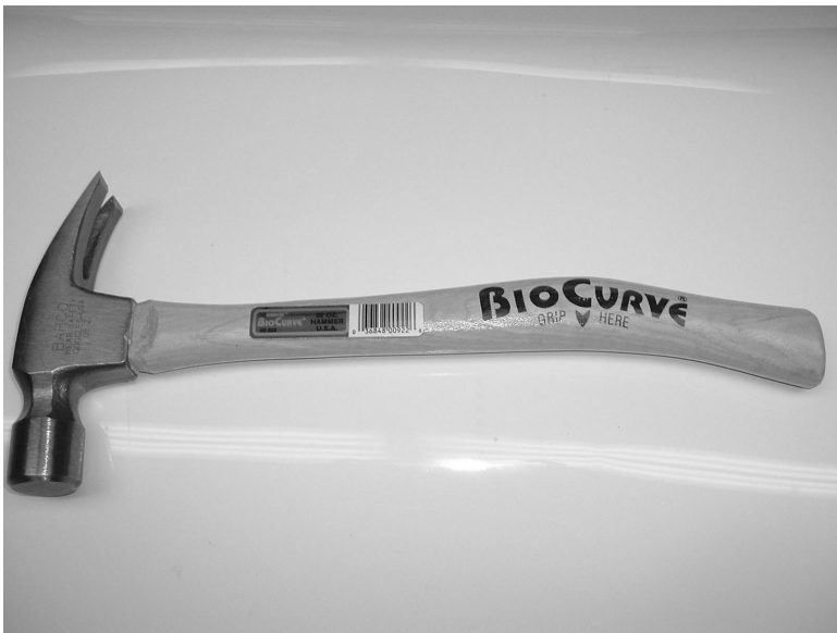
Figure 13-19. Examples of bent handles compared with a straight handle. (a) A conventional hammer handle that requires significant ulnar deviation of the wrist. (b) A curved handle reduces ulnar deviation. (c) A rip hammer with a BioCurve handle. (d) A mallet with a Bio-Curve handle. (Photos of BioCurve tools provided by and used with permission of BARCO Industries Inc., Reading, PA.)
