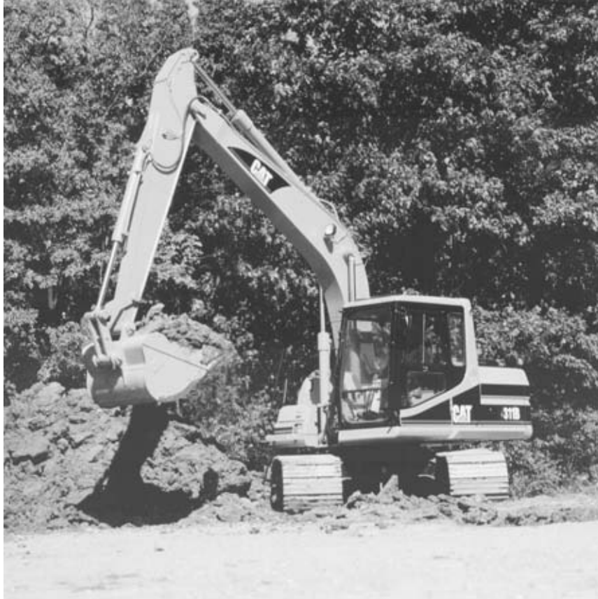
FIGURE 3-3 Backhoe (Permission granted by Caterpillar, Inc.).
