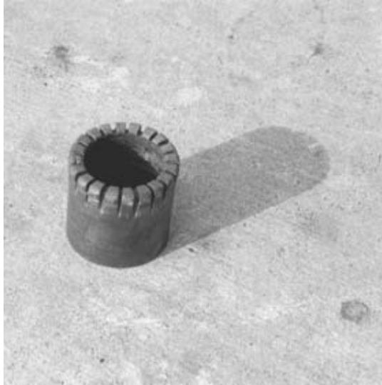
FIGURE 3-4 Cutting bit for rock coring.
