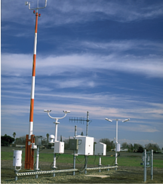
FIGURE 1–7 Gathering data is a basic part of the scientific method. This Automated Surface Observing System (ASOS) installation is one of nearly 900 in use for data gathering as part of the U.S. primary surface observing network. For more on ASOS, see Figure 12–4, p. 350. (Source: Bobbe Christopherson)
