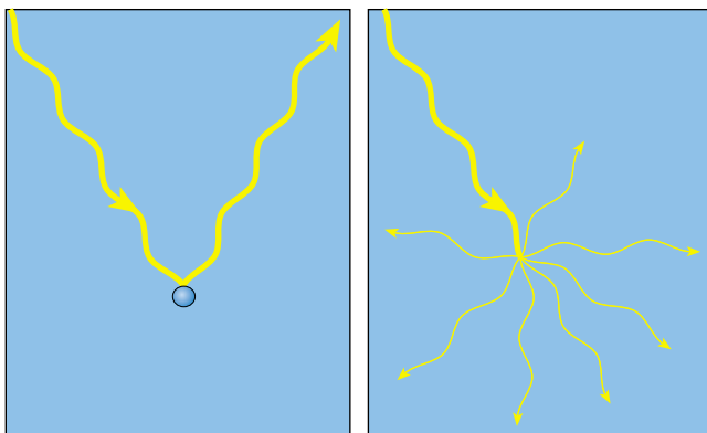
(a) Reflection (b) Scattering FIGURE 2-14 Reflection and scattering. (a) Reflected light bounces back from a surface at the same angle at which it strikes that surface and with the same intensity. (b) When a beam of light is scattered, it results in a larger number of weaker rays, traveling in all different directions. Usually more energy is scattered in the forward direction than is backscattered.
