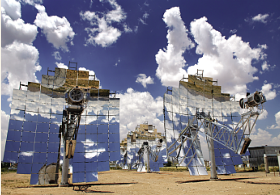
FIGURE 2-G A proposed solar facility near Los Angeles will consist of a 20,000-dish array using Stirling dish technology. (Photo by Randy J. Montoya/Sandia National Laboratories)
