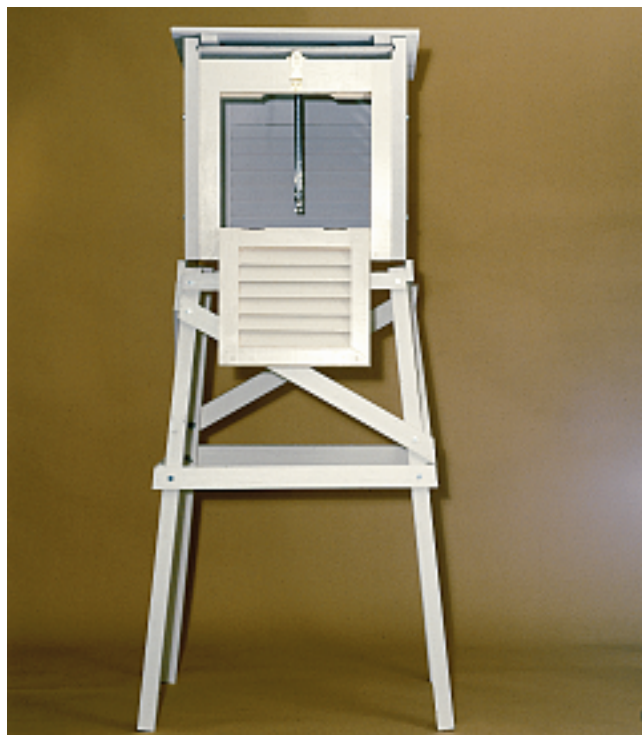
FIGURE 3-25 This traditional standard instrument shelter is white (for high albedo) and louvered (for ventilation). It protects instruments from direct sunlight and allows for the free flow of air. (Courtesy of Qualimetrics, Inc.)
