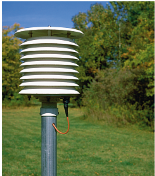
FIGURE 3-24 This modern shelter contains an electrical thermometer called a thermistor . (Photo by Bobbé Christopherson)
