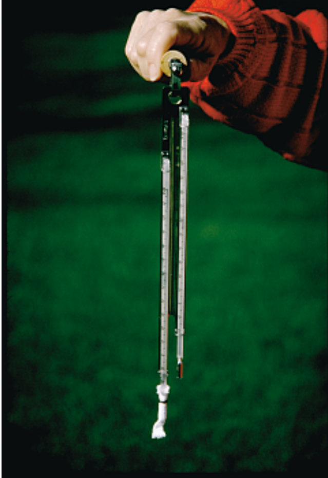
FIGURE 4-15 Sling psychrometer. This instrument is used to determine relative humidity and dew point. The dry-bulb thermometer gives the current air temperature. The thermometers are spun until the temperature of the wet-bulb thermometer (covered with a cloth wick) stops declining. Then both thermometers are read, and the data are used in conjunction with Tables C-1 and C-2 in Appendix C. (Photo by E. J. Tarbuck)
