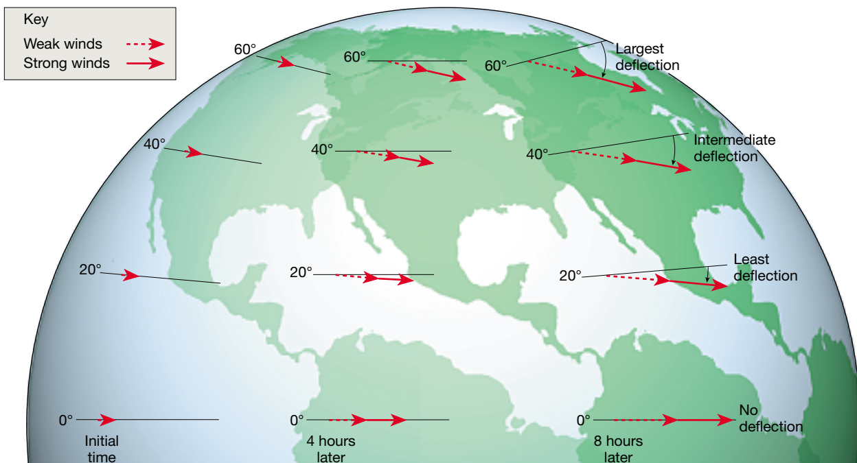
FIGURE 6-13 Coriolis deflection of winds blowing eastward at different latitudes. After a few hours the winds along the 20th, 40th, and 60th parallels appear to veer off course. This deflection (which does not occur at the equator) is caused by Earth's rotation, which changes the orientation of the surface over which the winds are moving.
