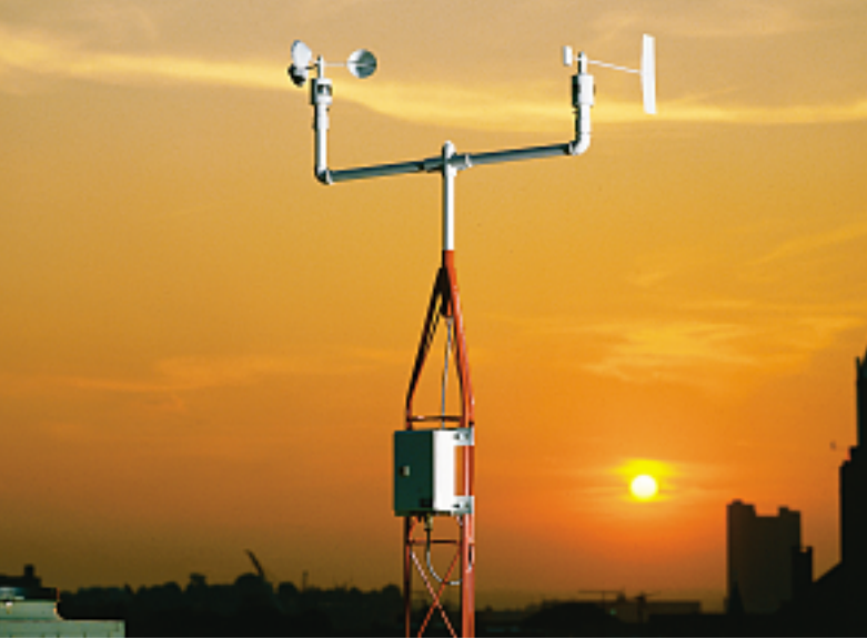
FIGURE 6-24 Wind vane (right) and cup anemometer (left). The wind vane shows wind direction, and the anemometer measures wind speed. (Photo by Belfort Instrument Company)
