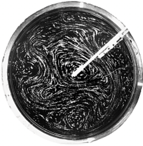
FIGURE 7-20 Photograph obtained from a dishpan experiment. The pan is heated around the edge to represent the equator, and the center is cooled to duplicate the poles. When the pan is rotated, a wavy flow develops with eddies embedded between meanders, as shown. This flow pattern closely parallels that produced in the “real” atmosphere, where the meanders represent the wavy flow of the westerlies and the eddies are cyclonic and anticyclonic systems embedded within this larger circulation. (Courtesy of D. H. Fultz, University of Chicago Hydrodynamics Laboratory)
