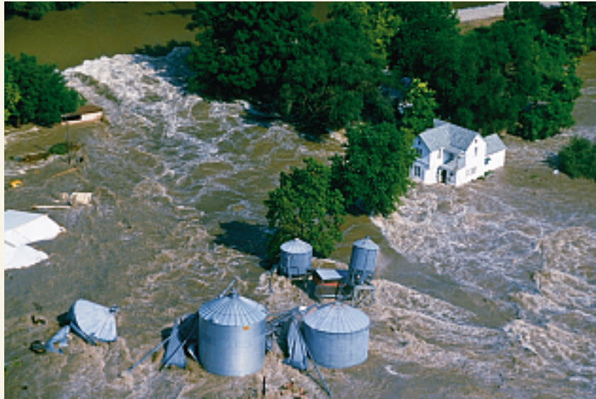
FIGURE 9-B Water rushes through a break in an artificial levee in Monroe County, Illinois. During the record-breaking 1993 Midwest floods, many artificial levees could not withstand the force of the floodwaters. Sections of many weakened structures were overtopped or simply collapsed. (Photo by James A. Finley/AP/Wide World Photos)
