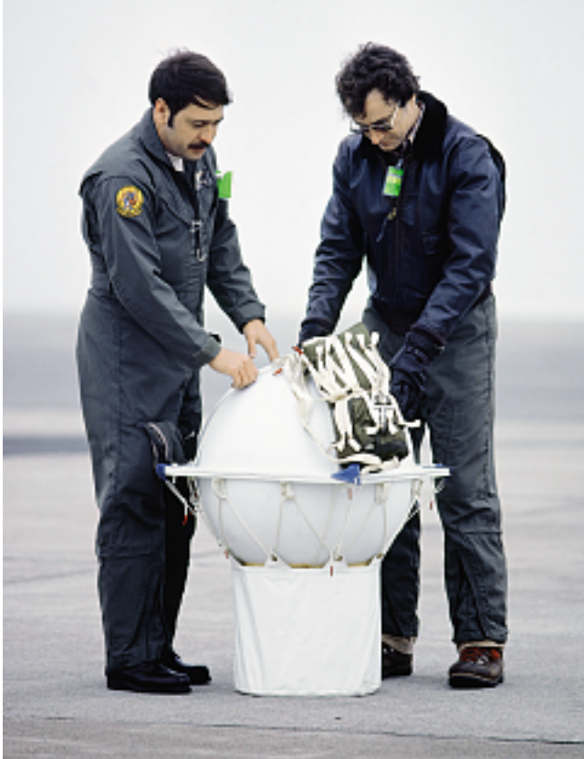
FIGURE 12-3 Data buoy used to record atmospheric conditions over a section of the global ocean. These data are transmitted via satellite to a land-based station. (Photo by Matthew Neal McVay/Stock Boston)
