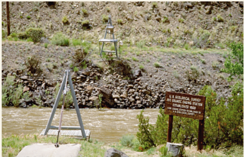
FIGURE 15-H One indicator of hydrological drought is significantly diminished streamflow. Continuous records of streamflow are collected by the U.S. Geological Survey at more than 7000 gauging stations in the United States. This station is on the Rio Grande, south of Taos, New Mexico. (Photo by E. J. Tarbuck).
