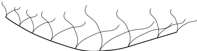
Figure 9.11: Nine Cross Sections of a Boat.
