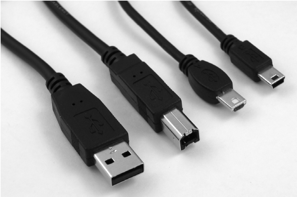
Figure 2-1: USB cable plugs from left to right: series-A, series B, mini-A, and mini-B.
