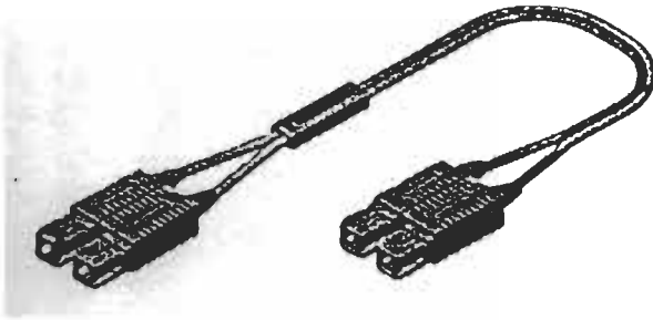
Fig. 4.7 Mode conditioning patch cable (MCP). The small box just behind one connector contains the offset ferrules; the transmit fiber from the optical transceiver is singlemode, all other fibers are multimode.
