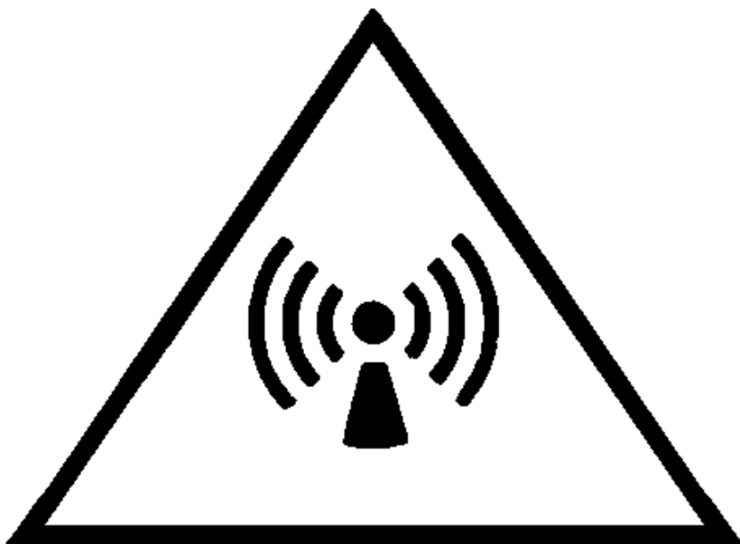
Figure 7.1 RF radiation safety warning sign
