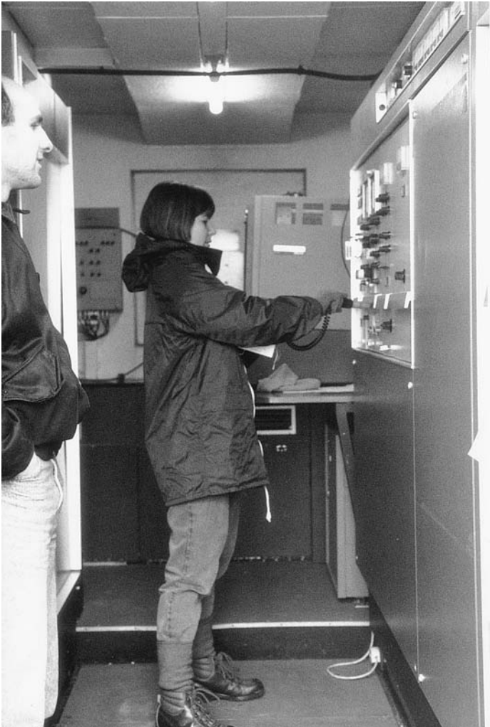
Figure 10.1 X-ray leakage measurement in a radar cabin during training
