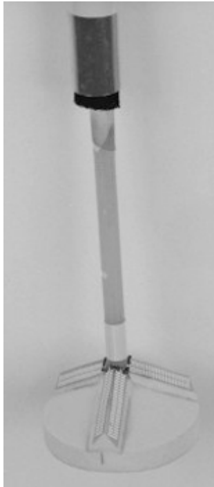
Figure 7.7 Actual electric field antenna – sensor structure for higher frequencies (Courtesy Narda Safety Test Systems)
