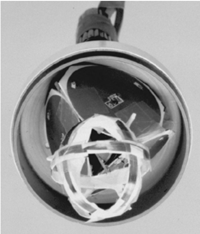
Figure 7.8 Actual magnetic field antenna – sensor structure (Courtesy Narda Safety Test Systems)
