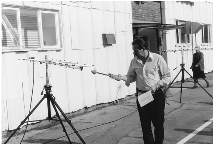
Figure 12.1 Yagi antenna fed by 100 W source for training exercises (Courtesy TUV Fareham)
