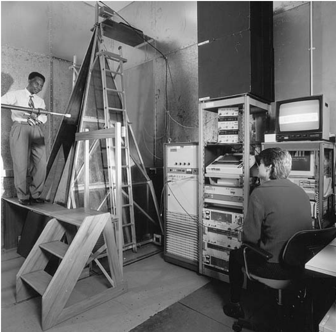
Figure 12.3 NPL tapered TEM cell for calibration in the range 180 MHz to 2.4 GHz (© Crown copyright 1998 reproduced by permission of the controller, HMSO)
