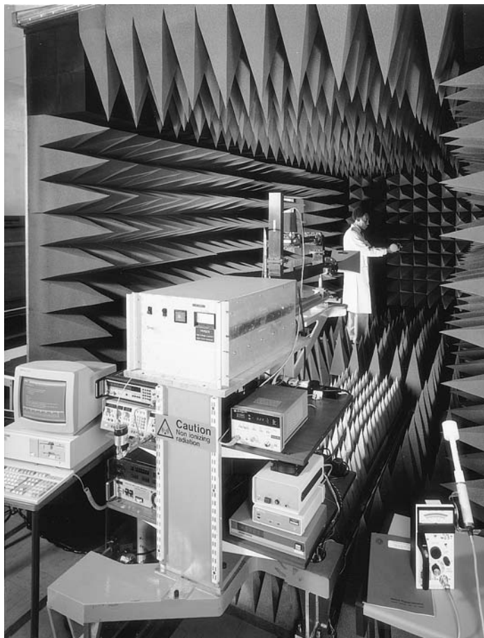
Figure 12.4 Anechoic chamber for calibration in the range 2.4 to 45.5 GHz (© Crown copyright 1998 reproduced by permission of the controller, HMSO)
