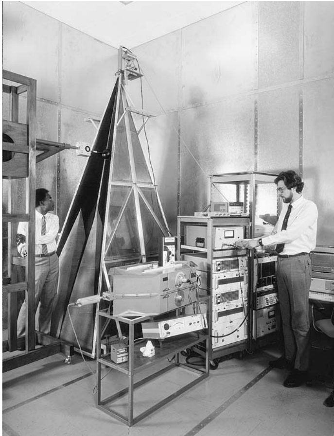
Figure 12.2 TEM cells used for calibration in the range 3 kHz to 2.4 GHz (© Crown copyright 1998 reproduced by permission of the controller, HMSO)
