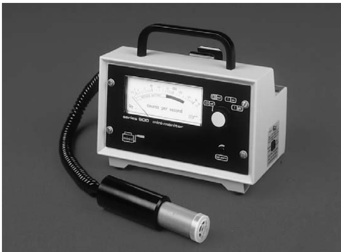
Figure 8.14 Mini-monitor type X radiation meter designed for finding X-ray and gamma radiation leaks (Courtesy Mini-instruments Ltd)
