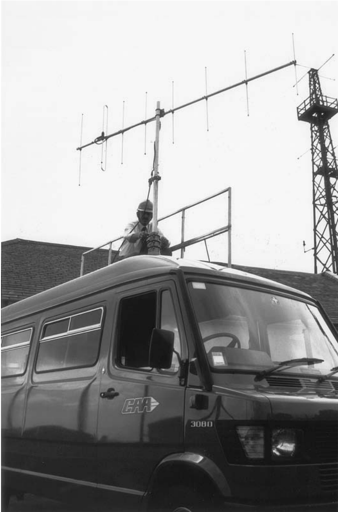
Figure 6.3 National Air Traffic Service technical investigation vehicle (Courtesy of NATS UK)
