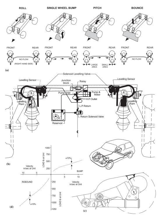
**Fig. 8.17** Hydragas suspension: (a) interconnection system; (b) automatic levelling system; (c) small car subsystem; (d) operating characteristics.
