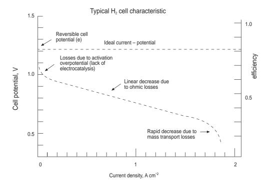
Fig. 4.2 Voltage/current relationship for hydrogen/oxygen cell.
