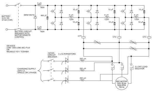
Fig. 1.12 Electric vehicle 45 kW inverter.
