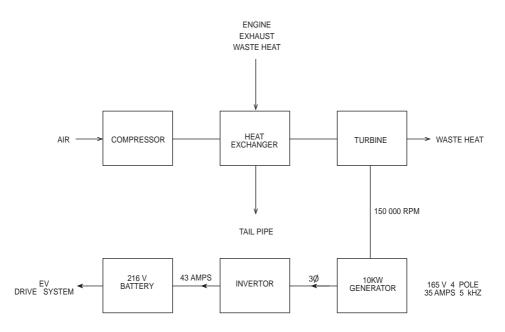
Fig. 2.21 Block diagram of turbine waste heat.
