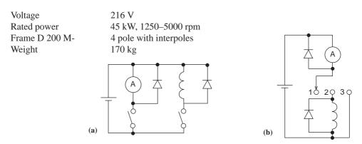
Fig. 3.15 Field windings: (a) shunt field machine; (b) 3 state strategy for series field machine.
