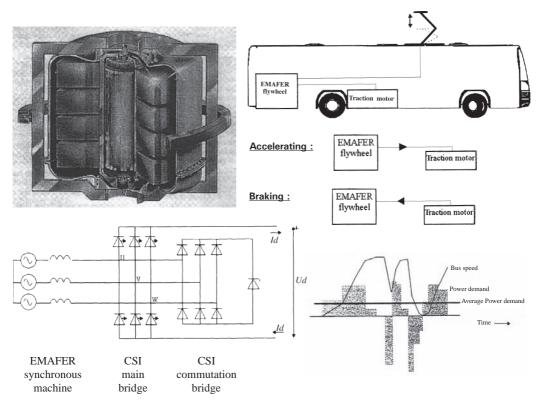
Fig. 6.12 Flywheel motor/generator: (a) Emafer flywheel/generator construction and electronic control; (b) power converter: shaded areas show power the Emafer has to supply/extract for accelerating or braking.
