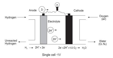
Fig. 4.1 Basic chemical reactions in a fuel cell.
