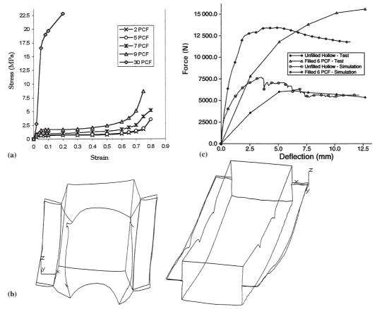
Fig. 7.2 Foam-filled tube behaviour: (a) Stress/strain curves for different density foams; (b) distorted shape for unfilled, left, and filled, right, structure; (c) deflection curves for unfilled and filled tubes.
