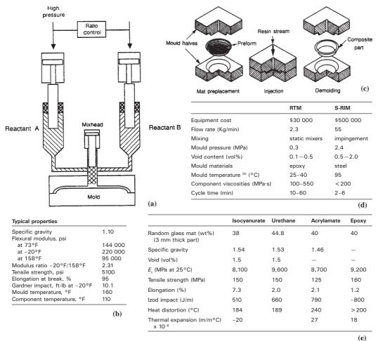
**Fig. 7.3** RIM process and properties: (a) RIM machine; (b) body-panel RIM formulation; (c) steps in the S-RIM process; (d) S-RIM and RTM compared; (e) S-RIM-composite properties.
