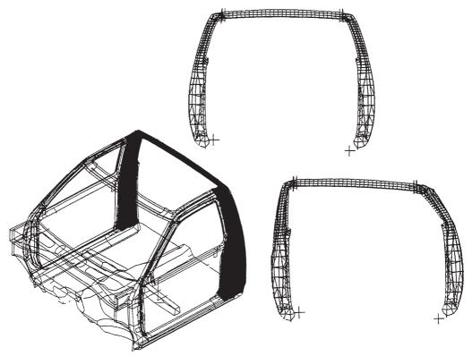
Fig. 8.14 FE model and B-pillar ring normal and deformed.
