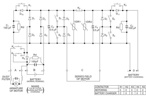
Fig. 3.18 Full circuit diagram of combined chopper/battery charger.
