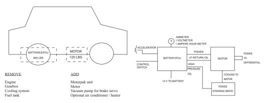
Fig. 1.25 Motorpak concept.
