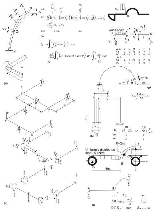
**Fig. 8.8** Stiff-jointed frames: (a) unit-load method; (b) seat support bearer; (c) unit-load calculation; (d) element subject to twisting and bending; (e) portal frame under combined loading; (f) loads in members; (g) semi-circular arch member under load: (h) front-end frame as portal; (i) battery-tray adjacent to wheel arch.
