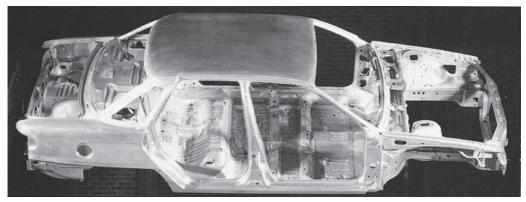
Fig. 0.1 Alcan's use of 5754 aluminium alloy substituted for steel in the Ford Taurus/Sable saved an impressive 318 kg. The client's constraint of minimal changes to the passenger compartment and use of existing production equipment must have constrained the possibilities for further weight reduction, however.
