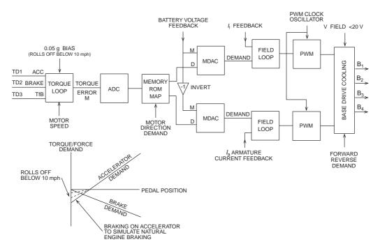
Fig. 3.19 Control system in motoring mode.
