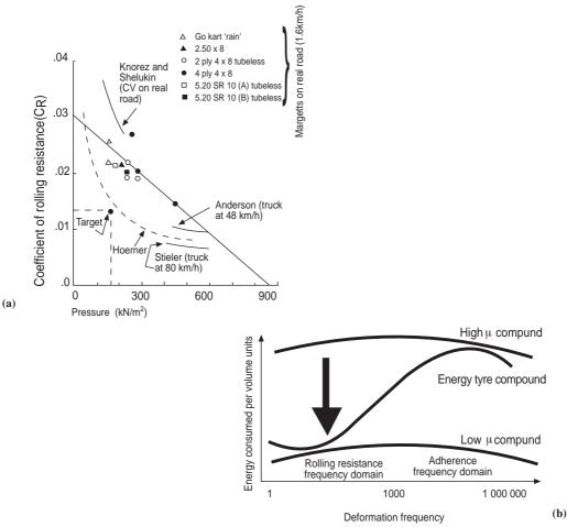
Fig. 8.25 Rolling resistance for small-wheeled and specialist tyres: (a) small tyres; (b) Michelin Energy tyres.
