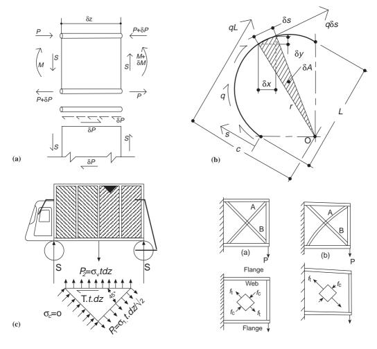
**Fig. 8.3** Thin-walled structural idealizations: (a) flat shear panels and end-load bars; (b) shear flow in curved section beam; (c) tension field in sidewall to examine shear buckling.
