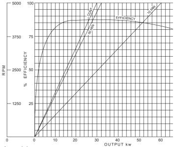
Fig. 3.2 N180L motor characteristics.
