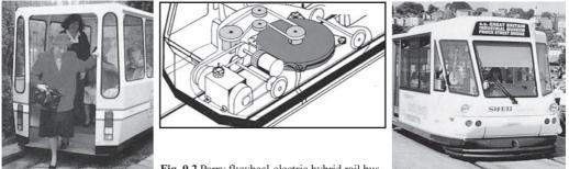
Fig. 0.2 Parry flywheel-electric hybrid rail bus.
