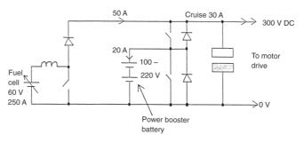
Fig. 1.9 Fuel-cell power conversion.
