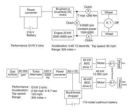
Fig. 1.7 A 45 kW parallel hybrid and 90 kW series hybrid.
