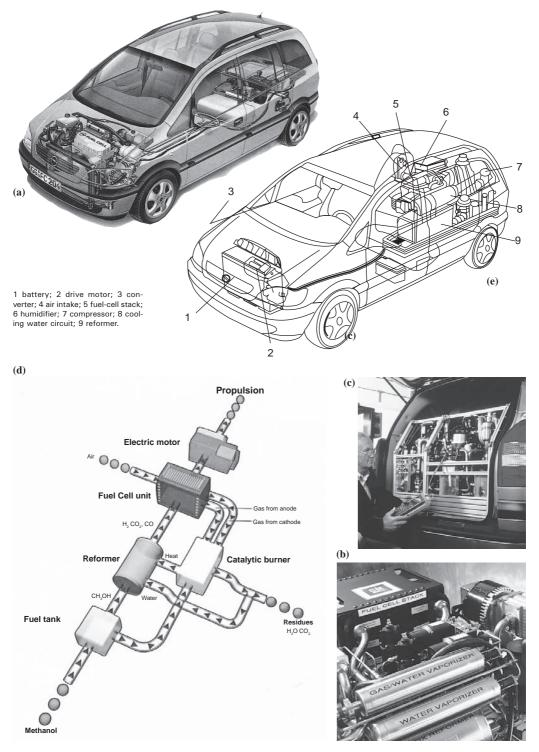
**Fig. 5.23** GM fuel-cell developments: (a) Zafira conversion package; (b) under-bonnet power-pack; (c) reformer and cells; (d) flow diagram; (e) latest package with on-board hydrogen storage.
