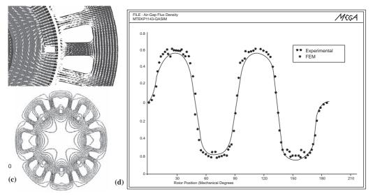
Fig. 3.10 Finite-element modelling: (a) the coupling meshes; (b) rotor at 45° from base; (c) air gap flux waveforms; (d) contour and vector flux.
