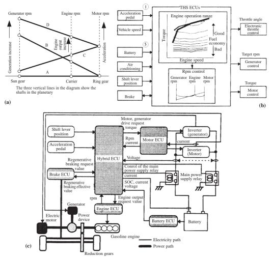
Fig. 6.15 Power-split control: (a) power interaction diagram; (b) THS control system; (c) ECU schematic.
