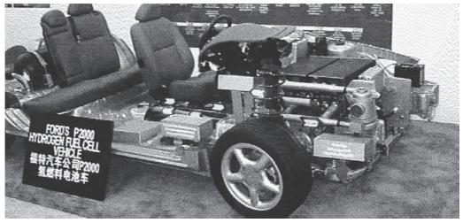
Fig. 5.24 Ford P2000 fuel cell platform with two 35 kW Ballard stacks.
