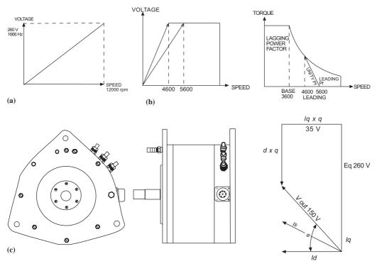
**Fig. 3.3** Example brushless motor characteristics: (a) no-load terminal voltage when machine is operated as a generator; (b) variation of machine terminal voltage with torque and speed (left) with variation of power factor with torque and speed (right); (c) vector diagram (right) of PMB DC motor (left), in field weakening condition 12 000 rpm no-load.
