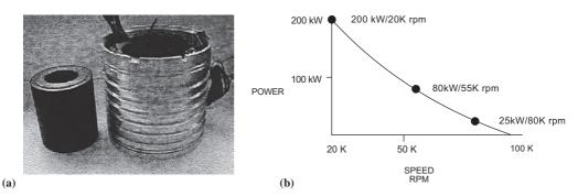
Fig. 3.7 Rotor design and machine performance: (a) a 150 kW, 20 000 rpm brushless DC stator-rotor; (b) power/speed for brushless DC motor with 3.5:1 constant power speed range.
