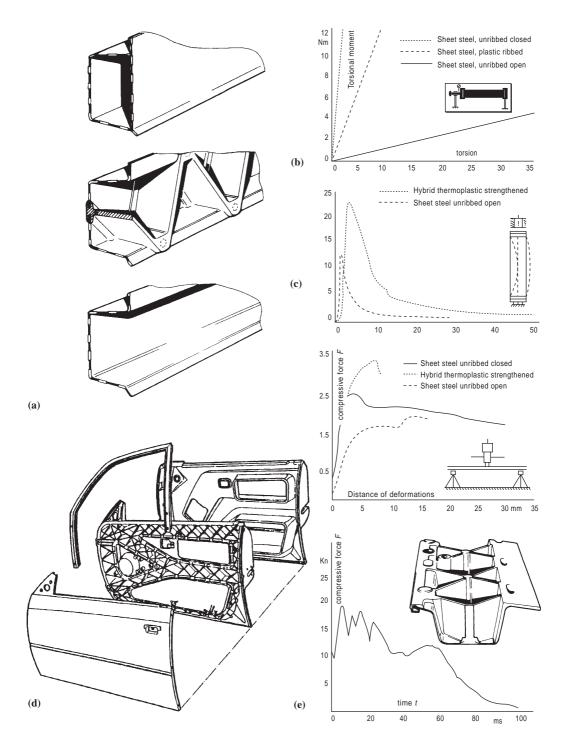
**Fig. 7.1** Hybrid metal–plastic beam: (a) test sections; (b) torsional stiffness comparison for three sections; (c) compression test results; (d) metal/plastic hybrid door structure; (e) interlocking connection panels for a door with impact pendulum test results on the assembly.
