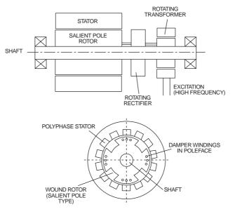
Fig. 3.13 Wound rotor synchronous machine with brushless exciter.
