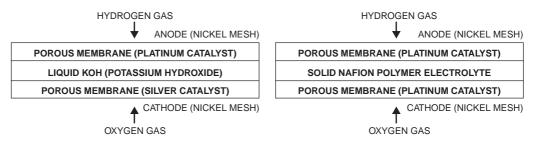
Fig. 2.13 Alkali (left) and PEM cell layouts compared.
