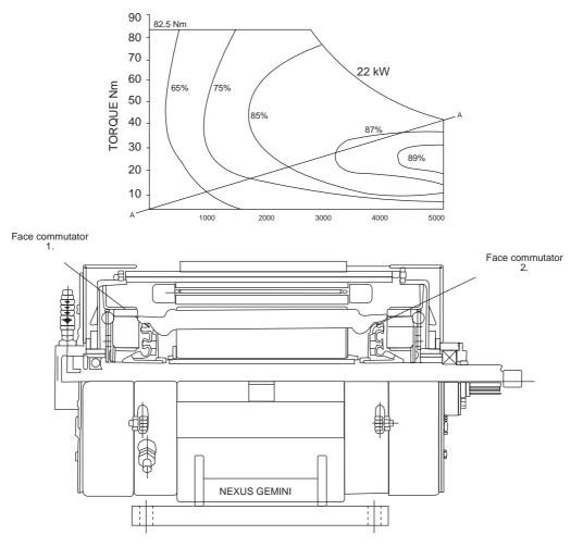
Fig. 1.14 Efficiency map and Gemini motor.
