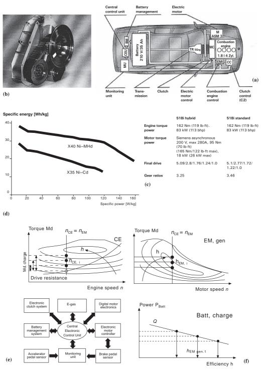
**Fig. 6.3** Map-controlled drive management: (a) BMW parallel hybrid drive; (b) parallel hybrid drive mechanism; (c) vehicle specification; (d) ragone diagram for the two battery systems; (e) vehicle management; (f) optimized recharge strategy.
