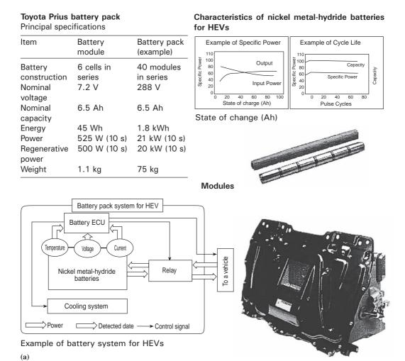
**Fig. 2.1** Production hybrid battery technologies compared: (a) Toyota Prius; (b) Sony/Nissan.
