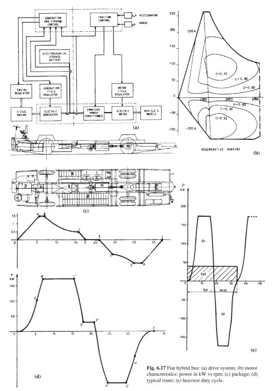
drive elements meant that considerable gains could be obtained in packaging the vehicle occupants. Using high power-density permanent-magnet motors driving the rear wheels allowed a particularly low floor of 12 in (305 mm) from the ground.
