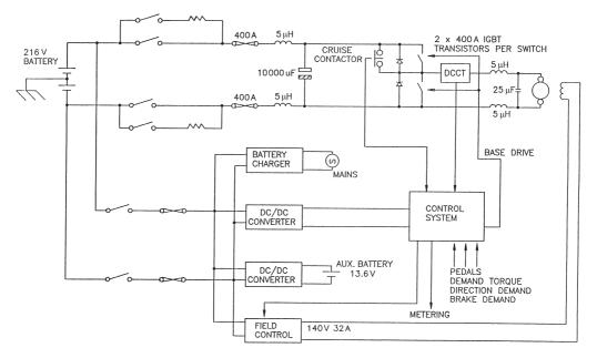
Fig. 1.11 Controller for 34 kW shunt field DC motor.
