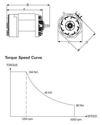
Fig. 3.14 Motor characteristics.
