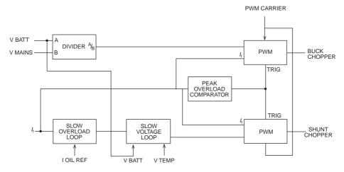
Fig. 3.20 Block diagram of battery charging controller.
