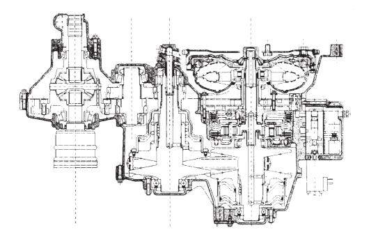
Fig. 8.21 Continuously variable transmission; the VDT P884 CVT.
