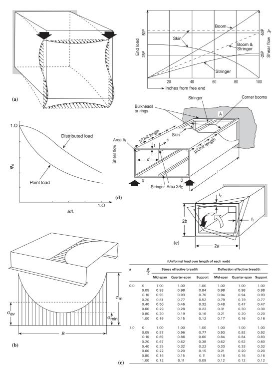
**Fig. 8.1** Box beams in bending and torsion: (a) axial warping of box beam in bending; (b) shear lag effect on breadth; (c) effective width ratios for simply supported box beams; (d) reinforced box beam with skin, stringer and boom load distribution above right supported box beams; (e) axial warping in torsion.
