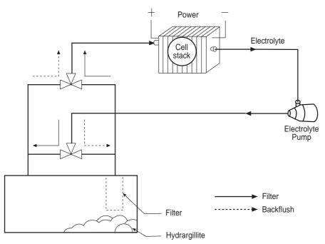
Fig. 2.6 Conceptual design of filter/precipitator system when integrated with aluminium/oxygen battery (courtesy Eltech Systems).
