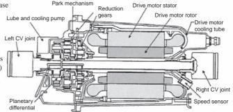
Fig. 5.21 Ecostar package, motor and specification.
