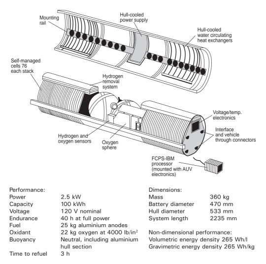
Fig. 2.9 Aluminium/oxygen power system and its characteristics (courtesy Alupower).
