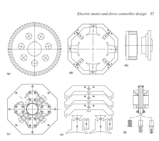
Fig. 3.1 Nexus II electric truck motor: (a) armature laminations; (b) faceplate adaptor; (c) brush holders; (d) segmented frame; (e) segmented yoke/pole assembly; (f) brush holder extrusions.
