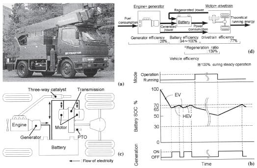
Fig. 6.21 Mitsubishi Canter-based hybrid municipal truck: (a) Complete package; (b) hybrid drive; (c) operating modes; (d) unit efficiencies.
