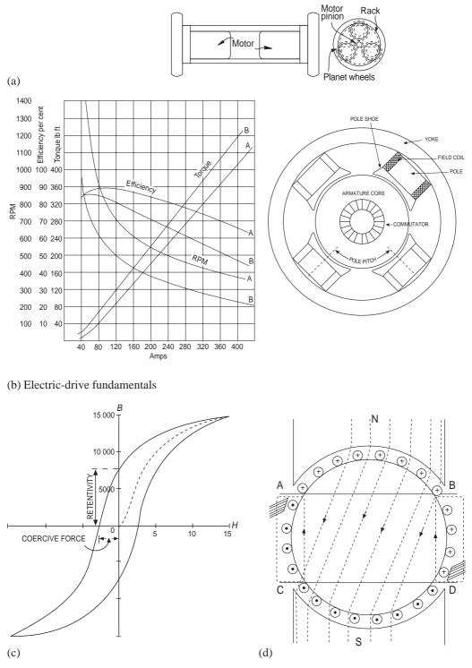
Fig. 0.4 Electric traction fundamentals: (a) Mercedes Electromobile motor; (b) motor characteristics; (c) hysteresis loop; (d) motor poles and their magnetic field.
