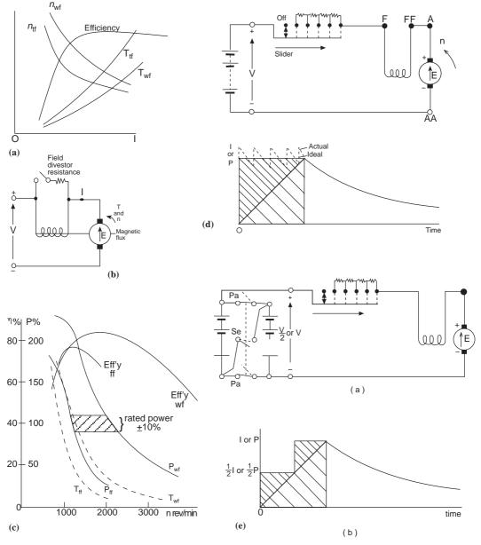
**Fig. 5.9.** Series-wound DC motor: (a) motor characteristics; (b) field diverter resistance; (c) speed-base motor characteristics; (d) rheostatic control; (e) parallel/series battery control.
