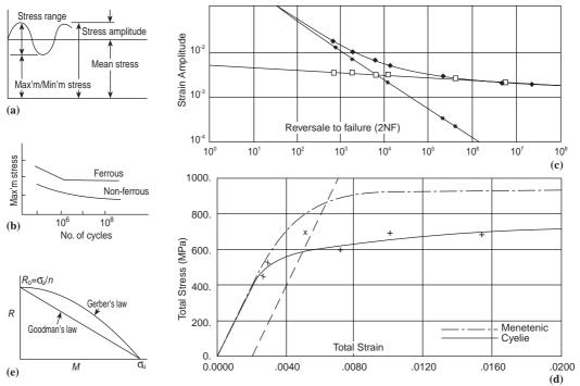
**Fig. 8.10** Fatigue life evaluation: (a) terminology for cyclic stress; (b) S–N diagram; (c) strain/life curves; (d) dynamic stress/strain curves; (e) fatigue limit diagrams.
