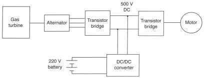
Fig. 1.18 Gas turbine technology.
