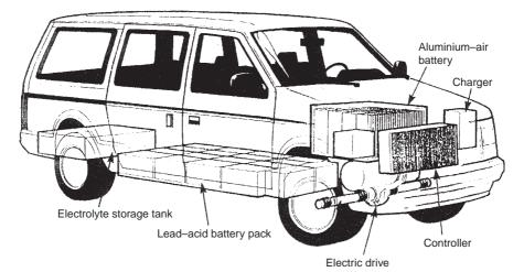
Fig. 2.7 A 6 kW range extender by Alupower, with lead-acid main battery.
