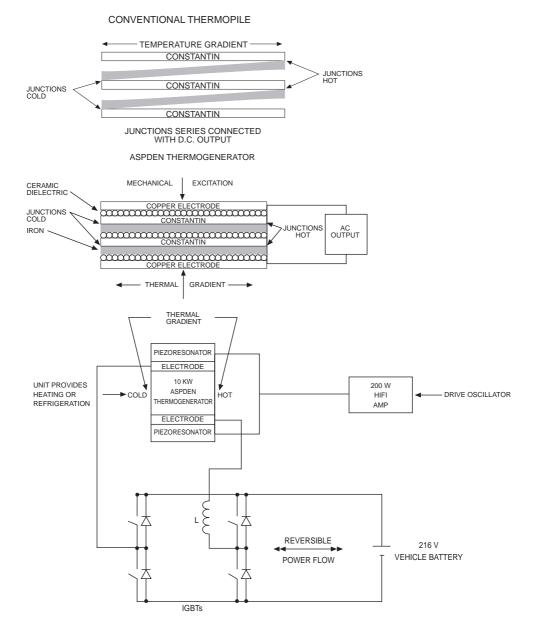
Fig. 2.23 Aspden thermogenerator and its control system (below).
