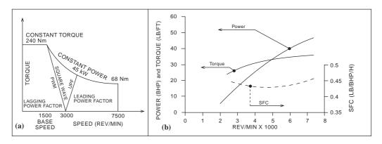
Fig. 6.7 System operation states (a), with performance curves of 300 cc fuel-injection Wankel engine (b).
