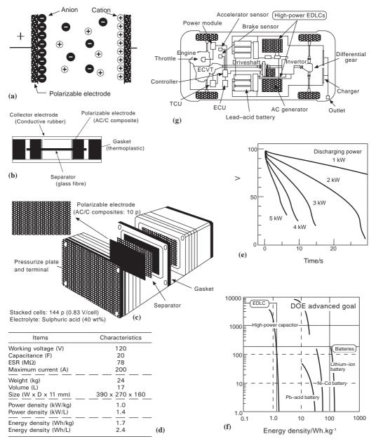
**Fig. 5.7** Supercapacitors: (a) EDLC model; (b) cell; (c) high-power EDLC schematic; (d) HP EDLC specification; (e) constant power discharge characteristics; (f) power density, *y*-axis in W/kg, vs energy density for high-power EDLC; (g) ELCAPA configuration.
