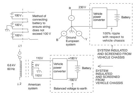
Fig. 1.5 Battery connections and earthing.
