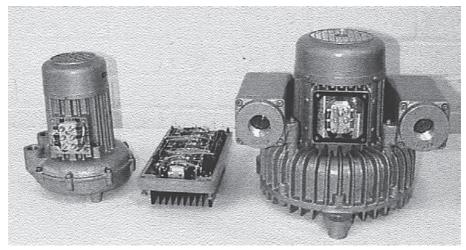
Fig. 2.16 Hydrogen/air blowers shown to left of drive electronics.
