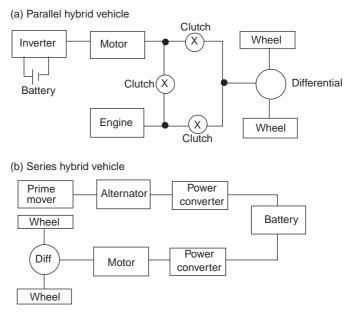
Fig. 6.1 Types of hybrid drive.
