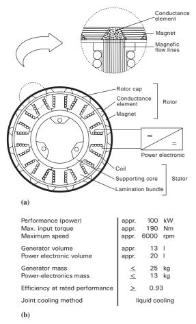
**Fig. 6.8** Advanced PM motor system: (a) trapezoidal iron conductors; (b) motor performance; (c) motor curves; (d) target performances.
