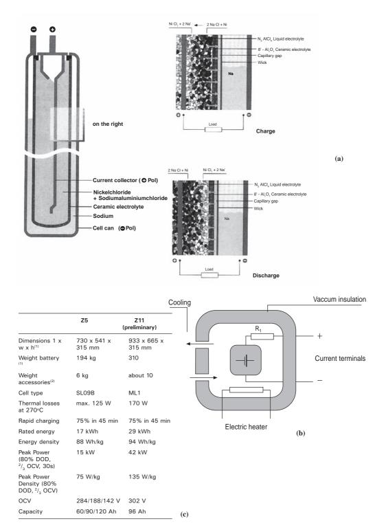
Fig. 5.4 ZEBRA battery: (a) cell; (b) cell-box; (c) performance comparison.
