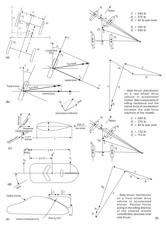
**Fig. 8.19** Traction vs stability; (a) ground-plane axis system; (b) lateral and central forces; (c) resolved aerodynamic forces; (d) forces on streamline body; (e) effect of rear fins; (f) graphical method.
