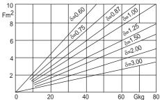
Alignment chart for the weight of steel sheets of different thicknesses. For small areas, 0-3 m<sup>2</sup>, a larger scale graph is used
