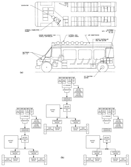
Fig. 6.18 Unique Mobility small hybrid bus: (a) Unique Mobility midibus; (b) power flow charts.
