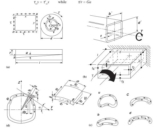
Fig. 8.2 Shear development in torsion: (a) shear in flat panel and circular section; (b) symmetrical and generalized box sections; (c) transition from closed to open section; (d) shear flows in beam element.
