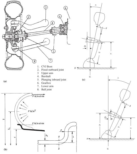
Fig. 8.23 Optimizing wheel design: (a) key elements to an independently suspended driven wheel; (b) element of rim section and tyre dimensions; (c) wheel disc analysis (static, top; cornering, bottom).
