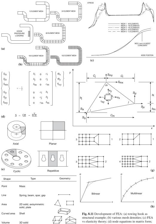
vs elasticity theory; (d) node equations in matrix form; (e) types of symmetry; (f) element shapes; (g) varying mesh densities; (h) stress-strain curve representation.
