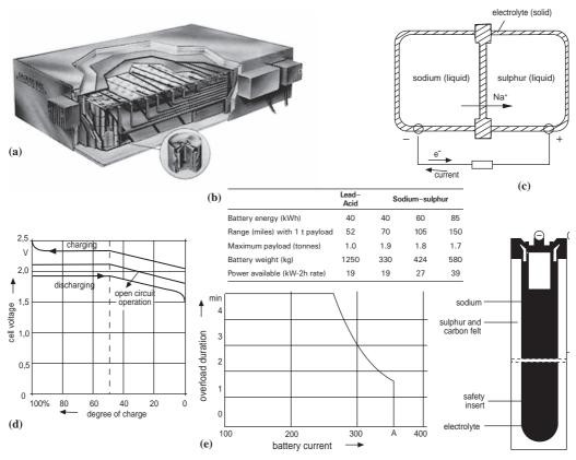
Fig. 5.2 Sodium–sulphur battery: (a) battery assembly; (b) projected performances; (c) ABB s-s cell; (d) energy capability; (e) overload capability.
