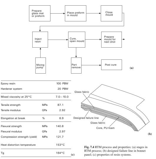
reinforcement for flat mouldings such as a bonnet may not be absolutely necessary. The handling of the fibre mats, however, can be difficult as they are rarely self-supporting. A bonnet can be designed as a slim sandwich structure instead of inner and outer mouldings. The rigid foam core thus provides a convenient method of supporting the fibre reinforcement during transportation of the fibre to the RTM mould, (b).
