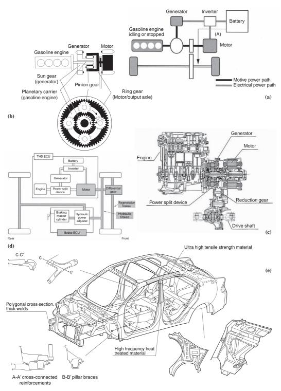
**Fig. 6.14** Prius systems: (a) THS schematic; (b) power-split device; (c) engine and hybrid transmission; (d) hybrid system in full-throttle acceleration; (e) lightweight structure detail.
