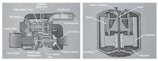
Fig. 5.8 Chrysler Patriot flywheel energy storage system: left, turbine; right, flywheel.
