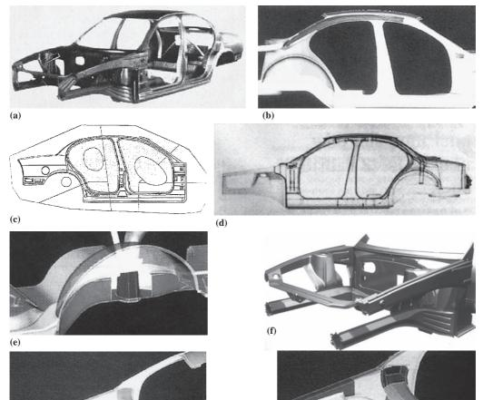
**Fig 7.12** ULSAB steel weight-reduction project: (a) body shell; (b) monoside panel; (c) hydroformed side roof rail; (d) principal application areas for bonding; (e) integration of rear shock absorber tower; (f) running the lower cowl through the A-pillar; (g) integration of front shock absorber tower.
