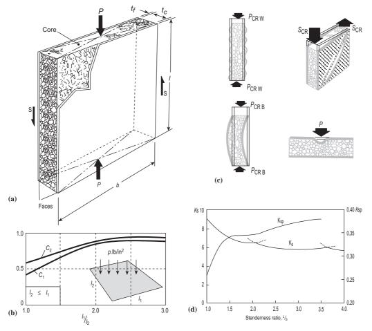
**Fig. 8.4** Foam-cored sandwich panels: (a) sandwich panel parameters; (b) correction factors; (c) failure modes; (d) *K* factors.
