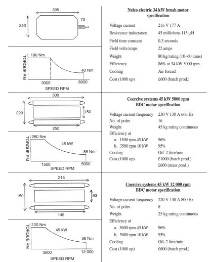
Fig. 1.10 Motor specifications.
