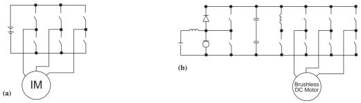
Fig. 1.22 (a) Single bridge inverter, (b) double chopper inverter.
