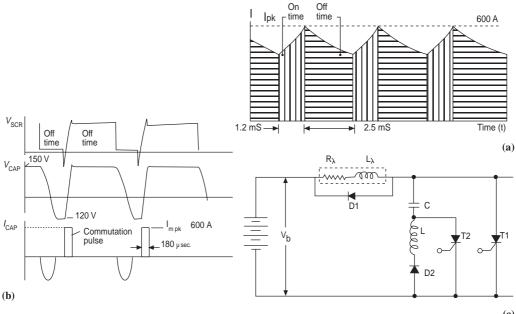
Fig. 5.20 Thyristor control: (a) controller pulses; (b) energy storage and reversal; (c) DC chopper circuit.
