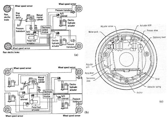
**Fig. 8.20** Electronic braking: (a) interaction of ABS, EAS and EMS; (b) electrohydraulic apply and rear braking systems; (c) Electric wheel brake.
