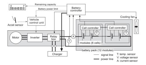
Fig. 5.6 Overall system configuration.
