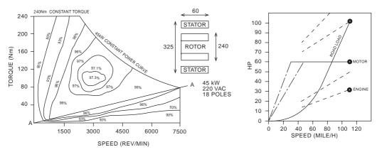
Fig. 6.6 Efficiency map, torque/speed curves and load matching.
