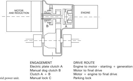
Fig. 6.5 The hybrid power unit.
