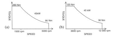
Fig. 1.8 Torque-speed curves for 45 kW vehicle (a) and each motor (b).
