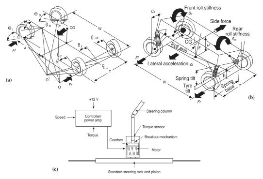
**Fig. 8.18** Suspension/steering geometry: (a) steer/slip angle; (b) front/rear roll stiffness; (c) Adwest electric steering system.
