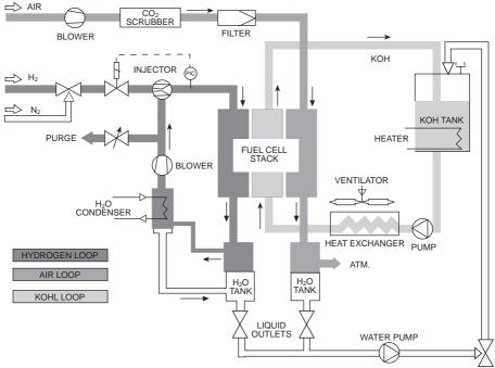
Fig. 2.14 Fuel-cell system schematic.
