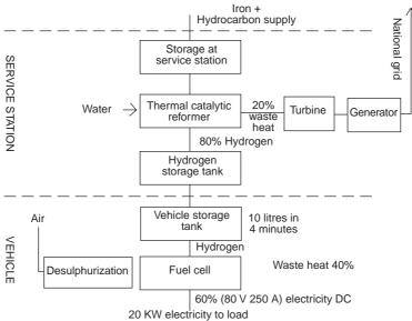
Fig. 1.3 Hydrogen distribution system.
