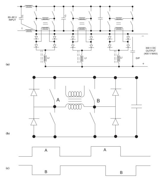
Fig. 2.19 Electronic system circuits: (a) DC/DC converter; (b) phase-shift chopper; (c) wave phase: full reinforcement (left) and 90° shift (right).
