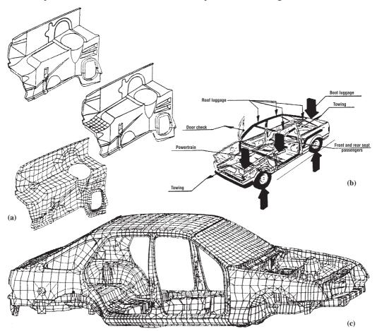
**Fig. 8.12** FEA of Ford car: (a) steps in producing FEA model; (b) load inputs; (c) global model for body-in-white (BIW).
