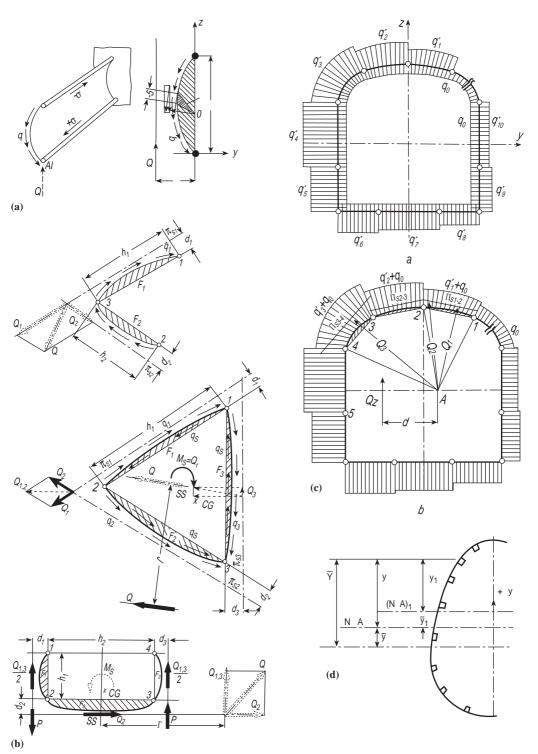
**Fig. 8.5** Curved shell structures: (a) idealization of curved panel; (b) shell made from curved panels; (c) multi-stringer shell beam; (d) reinforced generalized curved shell.
