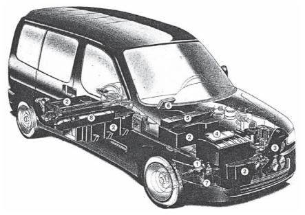
**Fig. 5.18** Citroen Berlingo Dynavolt: 1. electric motor and drive; 2. traction battery pack; 3. generator set; 4. motor controller; 5. generator controller; 6. drive programme selector; 7. LPG regulator; 8. LPG storage tank.
