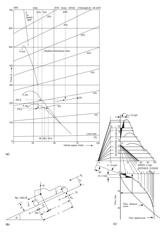
Fig. 8.16 Performance prediction: (a) tractive effort; (b) gradient resistance; (c) accelerative performance.
