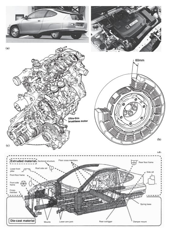
**Fig. 6.16** Honda Insight hybrid: (a) aerodynamic tailed body and underbonnet power unit; (b) motor; (c) motor installation; (d) body structure.
