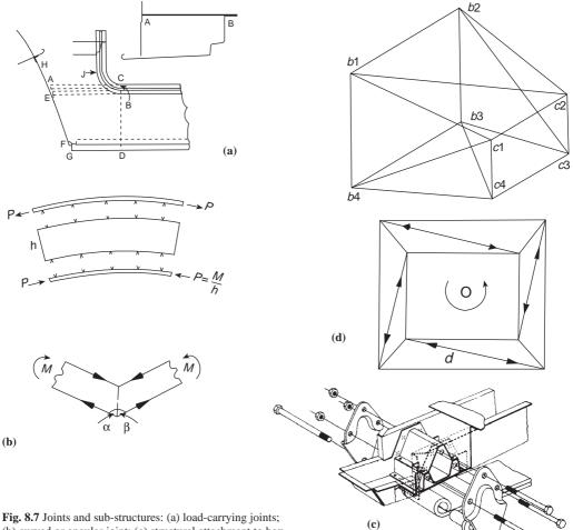
**Fig. 8.7** Joints and sub-structures: (a) load-carrying joints; (b) curved or angular joint; (c) structural attachment to box member; (d) single bay of space truss.
