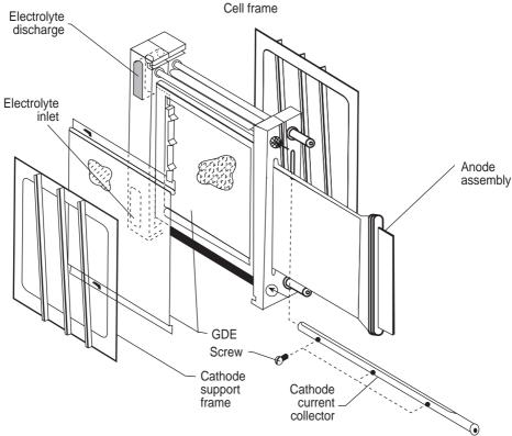
Fig. 2.5 Exploded view of aluminium/air bipolar battery (courtesy Eltech Systems).
