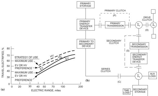
**Fig. 6.4** Justifying the hybrid: (a) EV traffic potential; (b) combined series–parallel mode.
