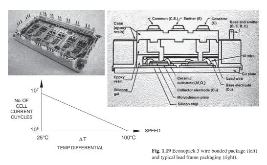
power silicon. New wire bond materials can offer a fatigue life of up to 10 million full current cycles with a Delta T of 25°C across the wire bond. The shorter pins on the package coupled with liquid cooling give best results. In Fig. 1.19, note that the temperature differential is the temperature difference between the connection pins and the baseplate in °C.
