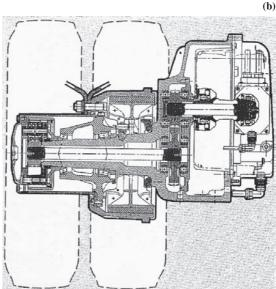
**Fig. 6.20** MAN/Voith concept city bus: (a) low floor package; (b) wheel motor; (c) controller; (d) drive characteristics.
