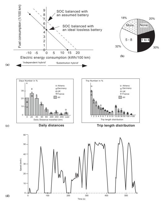
Fig. 6.2 HYZEM research programme: (a) characterizing a hybrid powertrain; (b) use of vehicle per day; (c) daily distances and trip lengths; (d) synthetic urban drive cycle.
