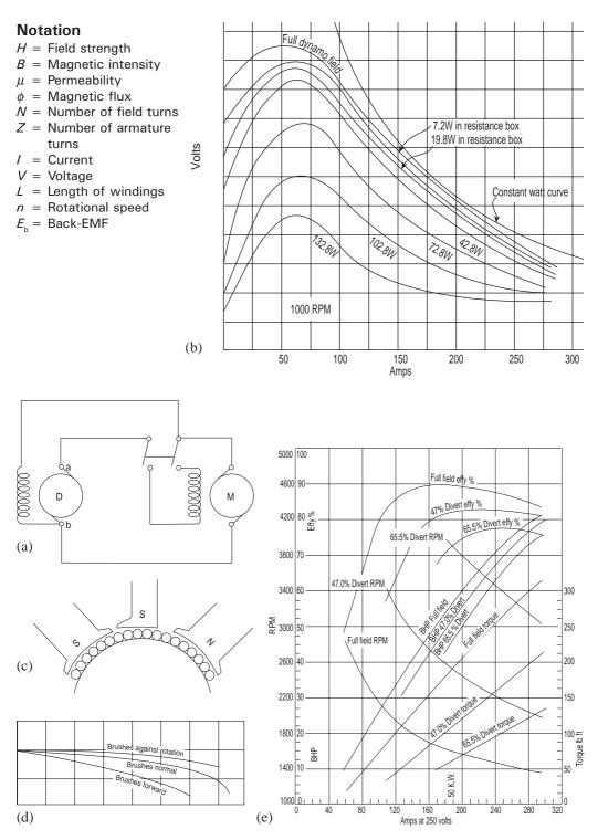
**Fig. 0.5** Electric transmission basics: (a) 'clutching' of electric transmission; (b) high EMF at low loads; (c) horned interpoles; (d) brush movement effect; (e) motor characteristics.
