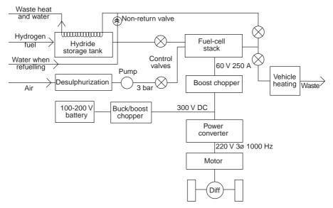
Fig. 1.4 Fuel-cell electric vehicle.
