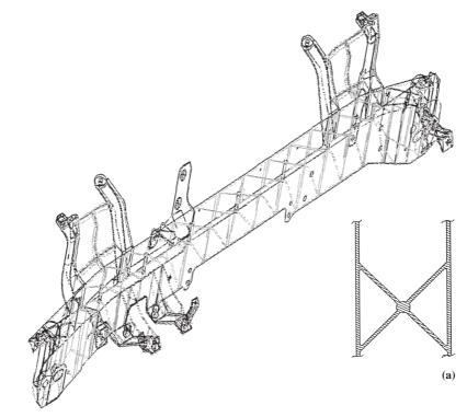
Fig. 7.14 Magnesium bulkhead crossmember: (a) open-section carrier beam; (b) multi-web section.
