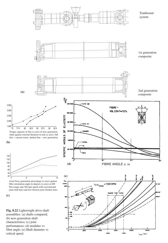
of a shaft, with  $0^{\circ}$  fibre orientation, is comparatively low; (e) is based on a realistic orientation of 15°. Usually multi-layer composites are involved and the elastic behaviour of any defined combination of layers is generally derived from the properties of one unidirectional layer, defined by the modulus parallel and perpendicular to the fibres, one of the two Poisson's ratios and the inplane shear modulus.
