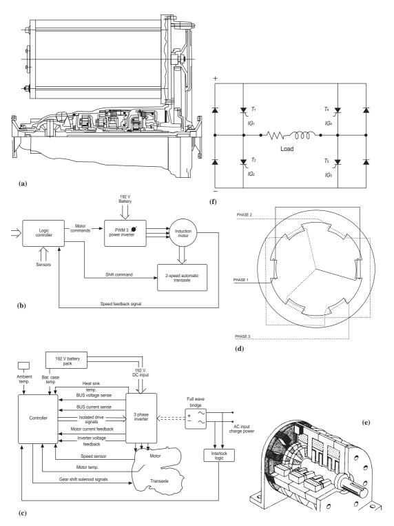
Fig. 5.16 AC drive systems: (a) transaxle motor; (b) controller arrangement; (c) controller drive system; (d) 3 phase induction motor stator; (e) air-gap type reluctance motor; (f) induction motor controller.
