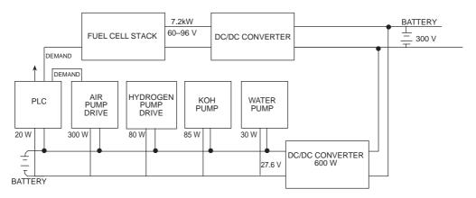
Fig. 2.15 Fuel-cell control system.
