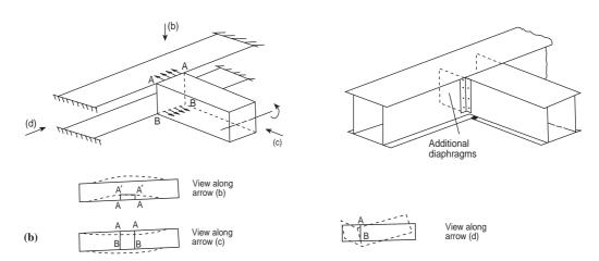
**Fig. 8.9** Panels and joints in box members: (a) effect of panel removal on box tube; (b) use of diaphragms at beam intersections; (c) B-post section; (d) neutral axis determination.
