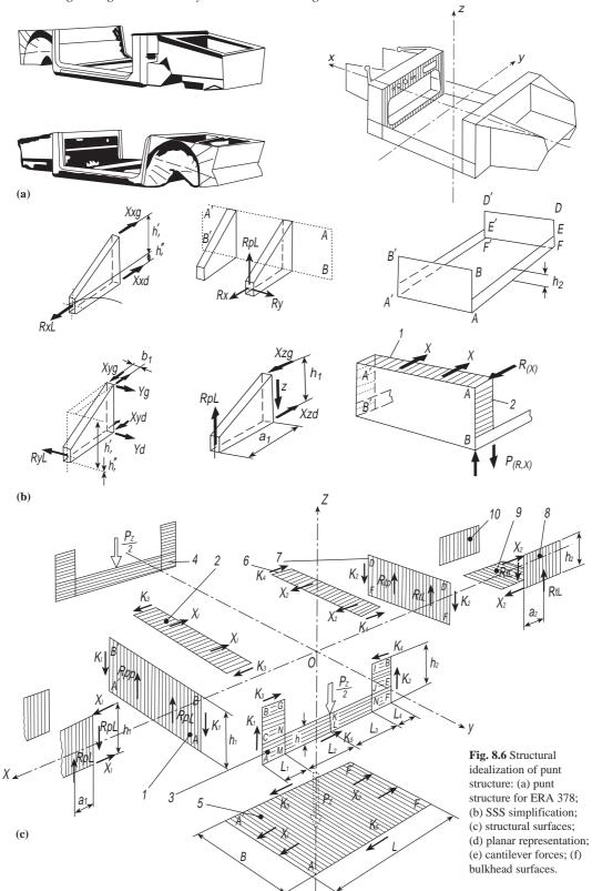
the use of large uniform-section box tube for the sills, A/C-posts and their upper and lower crossmembers. The use of a sandwich floor panel, with such a punt structure, would also allow central positioning of propulsion-battery packs in a structurally efficient manner for a mid-size electric car.
