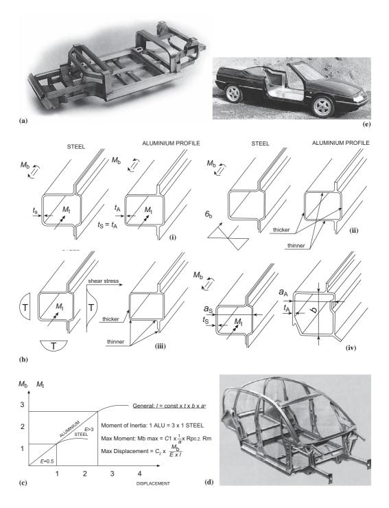
**Fig. 7.13** Aluminium alloy structures: (a) hydro aluminium structure; (b) sill section parameters when (i) straight substitution of aluminium for steel; (ii) optimized for bending; (iii) optimized for torsion; (iv) optimized for stiffness; (c) Applied moments vs displacement for sill member optimized for stiffness; (d)  $Al_2$  concept structure; (e) XMple concept car using aluminium skinned sandwich panels.
