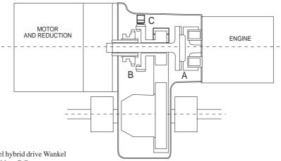
Fig. 2.20 Parallel hybrid drive Wankel engine and brushless DC motor.
