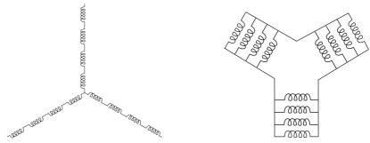
Fig. 3.11 Star, left, and parallel-delta, right, winding.
