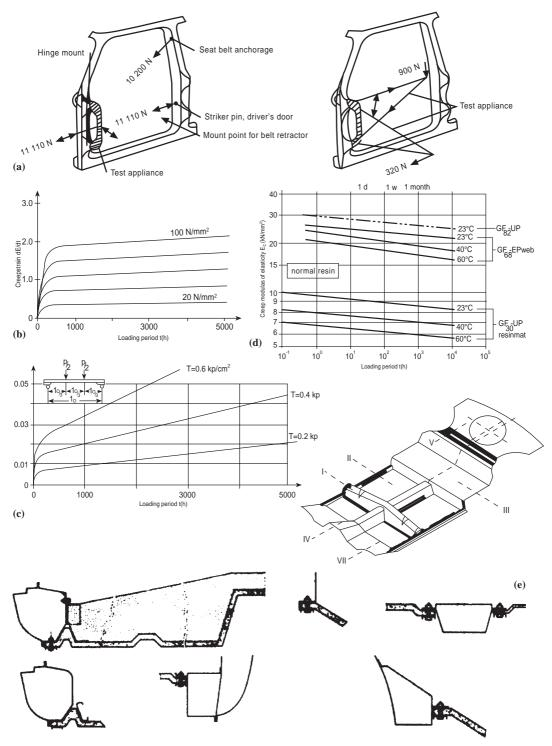
**Fig. 7.7** Composites in passenger cars: (a) test forces on front door frame; (b) creep strain of GRP showing exponential and linear regions; (c) creep of rigid PUR foam under constant shear; (d) time/temperature dependency of GRP; (e) composite GRP floor design.
