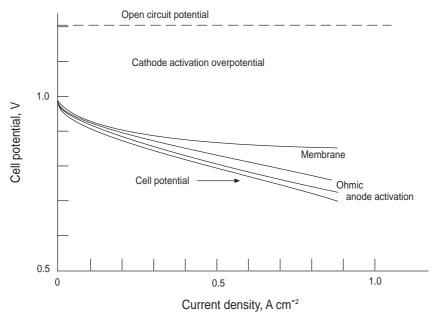
Fig. 4.3 SPFC characteristics.
