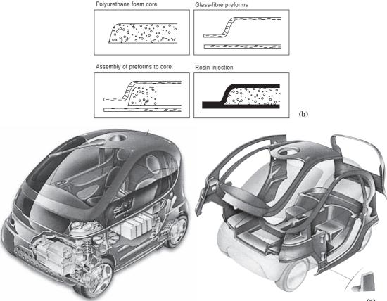
Fig. 7.5 Tulip concept car: (a) structure; (b) sandwich configuration.
