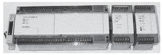
Fig. 2.18 Mitsubishi 80 I/O F-series PLC with DAC, ADC and RS232 modules.
