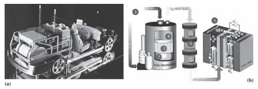
Fig. 5.25 Liquid hydrogen or reformed fuel: (a) Renault cryogenic storage; (b) Arthur D. Little reformer.
