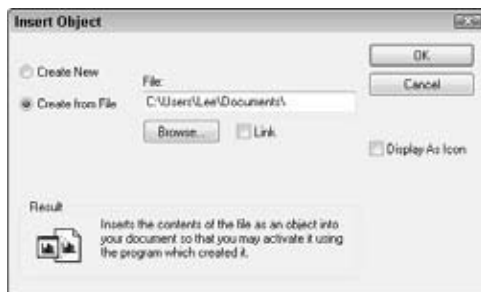
Figure 3-12: Attaching a file to a drawing other than a drawing, a DWF file, or an image.
