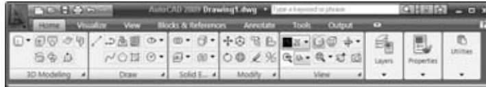
Figure 2-2: The ribbon gives you quick access to a variety of 3D-related tools.
