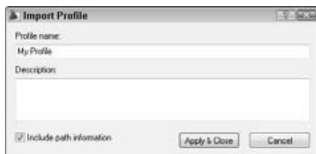
Figure 1-8: Profiles can be exported from AutoCAD and imported back in with the Import Profile dialog box.
