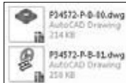
Figure 3-16: The markings on the bottom icon indicate that the drawing file has been digitally signed.
