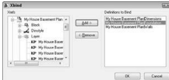
Figure 3-5: Xbind allows you to bind selected named objects into the parent drawing.
