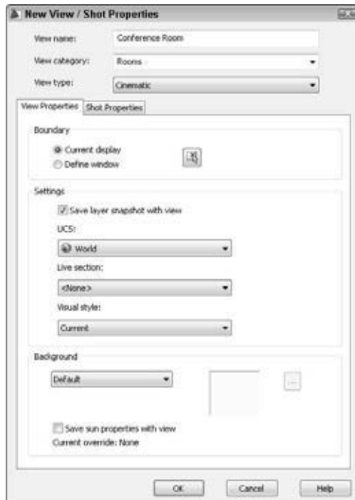
Figure 3-11: You use the New View/Shot Properties dialog box to create named views.
