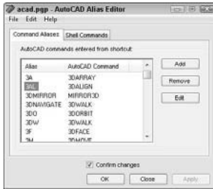
Figure 1-10: The Alias Editor dialog box assigns a new identity to a command.
