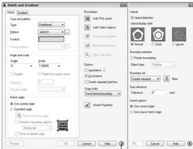
Figure 3-2: The Hatch and Gradient dialog box with the Hatch tab active and expanded.
