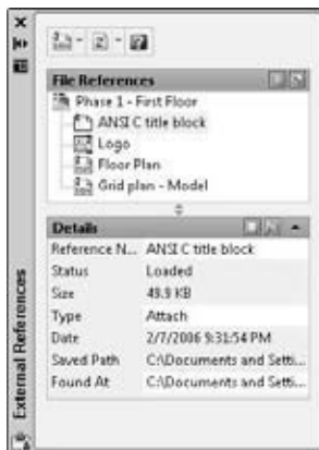
Figure 3-1: The External References palette is used to manage attached DWG, DWF, DWFx, DGN, and raster image files.
