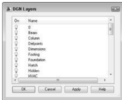
Figure 3-10: The layers for a DGN underlay are kept out of the parent drawing but can be accessed with the DGN Layers dialog box.
