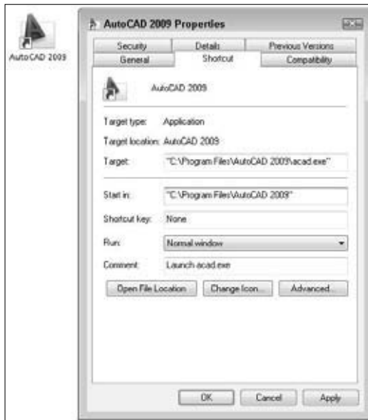
Figure 1-1: Use the Properties dialog box to alter the behavior of the shortcut.
