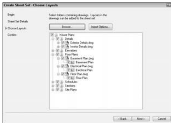
Figure 2-5: The tree view displays the folder structure and available layouts in drawings for import.
