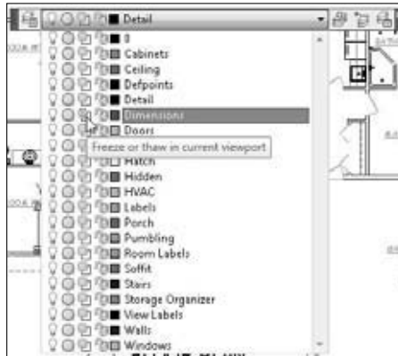
Figure 1-11: Freezing a layer in the current viewpoint.
