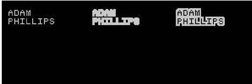
Figure 12.5: ilabel Output on Left, Dilation in Center, XOR of Both on Right
