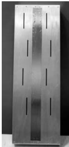
Figure 5.22 If we have to align our radiating elements along a surface of predefined shape (e.g., an aircraft fuselage) we may find slot antennas interesting. Here, an eight-element array is shown for the military L-band links.
