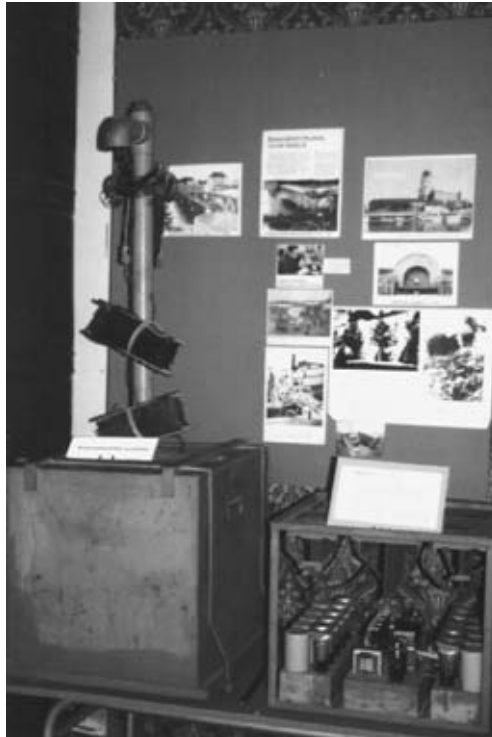
Figure 1.6 A radio system might easily fail even if its components are perfect. During World War II, these Russian radio-controlled mines all used the same carrier frequency and were easily jammed.
