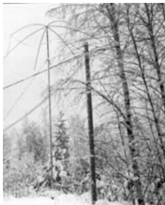
Figure 7.9 Seasonal variations of vegetation and soil affect the impedance of many HF antennas. So does snow, which may be wet or dry, depending on temperature.
