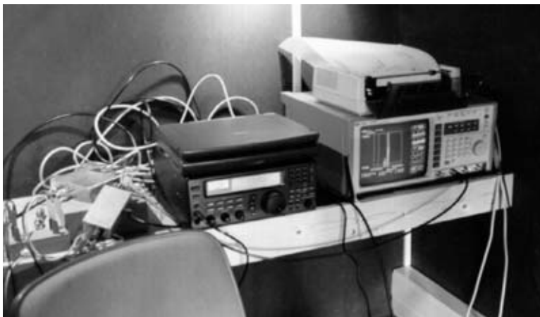
Figure 6.47 A view of the test vehicle interior with the time interval RX and the analyzer in the upper corner.
