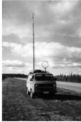
Figure 7.19 Airborne HF field strength measurements were supplemented and later replaced to a large extent by ground measurements, which were performed with a dedicated van. Note the loop antenna on the roof.
