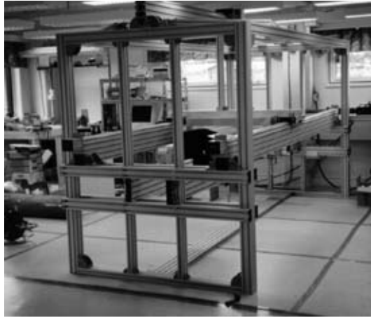
Figure 4.34 An example of a stable positioner for millimeter-wave laboratory work. The span is about 4m and positioning uncertainty less than 1 mm.
