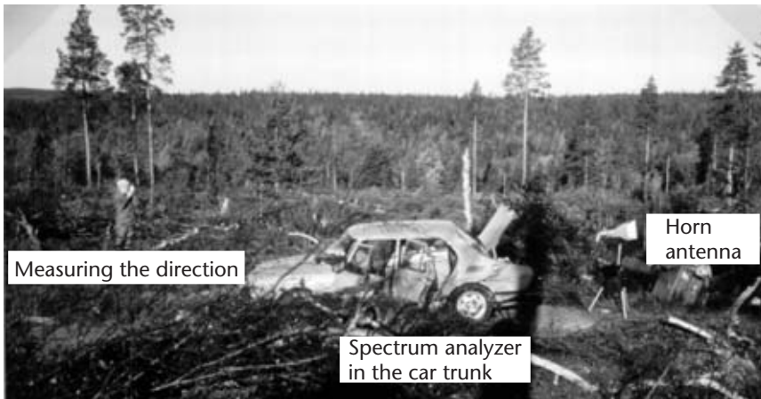
Figure 6.26 A typical isolated test site. The task at the time of photographing was to find the correct alignment for the receiving horn antenna.
