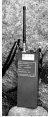
Figure 6.25 Similar in internal electronics to the maritime beacon, this dark gray TX was intended for military users.
