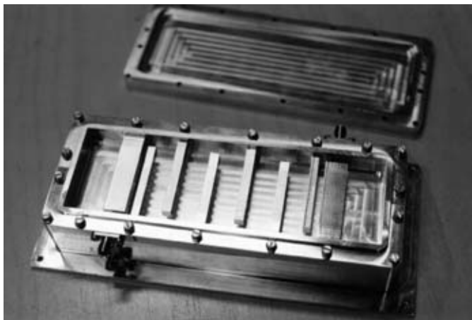
Figure 4.7 A high performance stripline bandpass filter for L-band radar. Completing this all-milled design from the announcement of system specifications took about 3 months.
