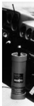
Figure 6.24 Due to delays in the 406-MHz frequency stabilization, a separate 121-MHz TX for the maritime users was assembled.
