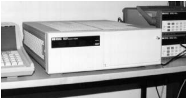
Figure 6.44 The most unreliable part of the test installation was the new commercial cesium clock, the prolonged repair of which caused a 4-month delay to field trials.
