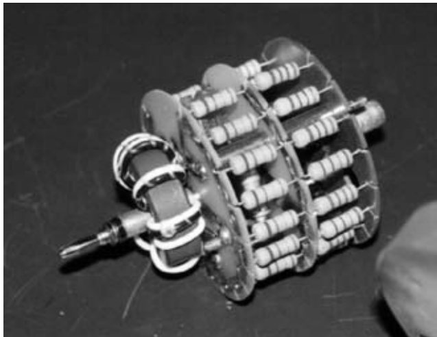
Figure 5.9 A very wideband matching of a monopole antenna is impossible with a lossless network. One commercial military VHF antenna includes a set of resistors as a questionable solution to the problem.
