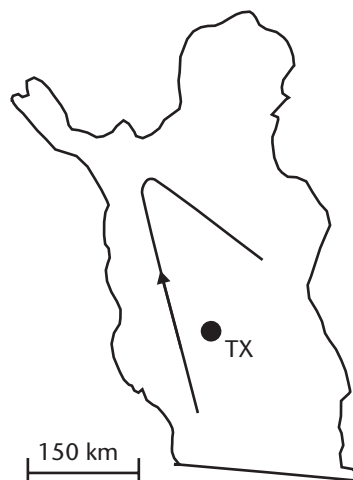
Figure 6.49 This radar plot shows the expected operating range obtained at 3,000m with just a simple ground plane antenna at the TX site.
