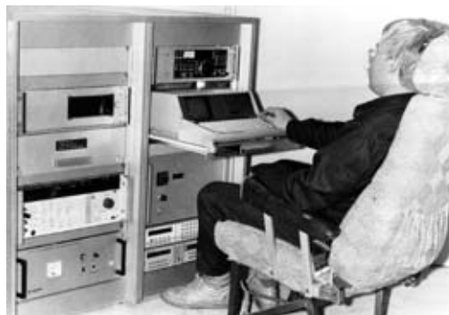
Figure 7.17 After successive upgrades and modifications, flight inspection system I was put into commissioning tests.
