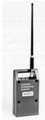
Figure 6.23 The prototype 121.5/406-MHz beacon. Overall size is about that of a shoebox. The UHF antenna is mounted inside the carrying handle, because the whole outer skin is of special ABS plastic. Lithium batteries fill most of the enclosure.
