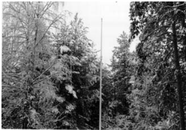
Figure 3.19 This installation had very few possibilities for competing with the interfering foreign transmission. Snow-covered trees absorbed part of the RF energy and caused frequent tuning difficulties. The antenna feeder is positioned incorrectly, too.
