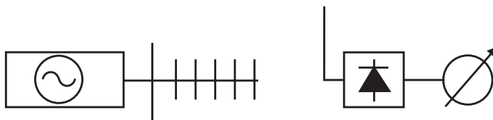
Figure 7.4 The block diagram of the whole measuring chain includes a VCO, an amplifier, a directional bridge, and a display. The propagation path is formed between a ground plane Yagi and a small monopole.
