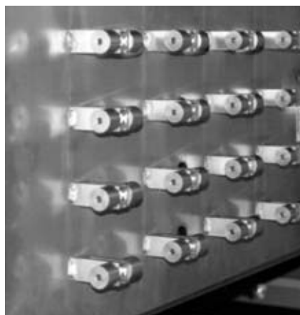
Figure 5.33 A part of the dipole array used for tests. The unfortunate feature of this construction is the high mutual coupling between adjacent rows, not better than -20 dB.
