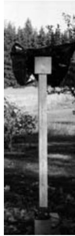
Figure 6.36 Calibration test target in the author's wife's garden. In this case an absorber plate was rotating around the rectangular zinc-bronze plate. Plastic bags provided a temporary weather shield.
