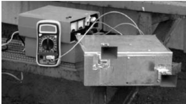
Figure 6.35 Prototype millimeter-wave radar hardware ready for first field trials. The unit uses a pulse width of 70 ns and has a measuring range up to 500m. Separate 20-dBi pyramidal horn antennas are used for transmission and reception.
