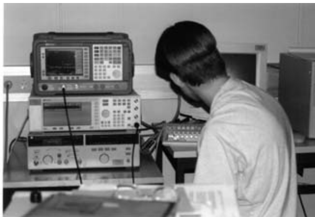
Figure 5.42 The author’s son is seen here tediously measuring the phase and amplitude patterns of a full array. Two microwave generators, a spectrum analyzer (the pile on the left), and a VNA (in the foreground and thus not visible) were used.
