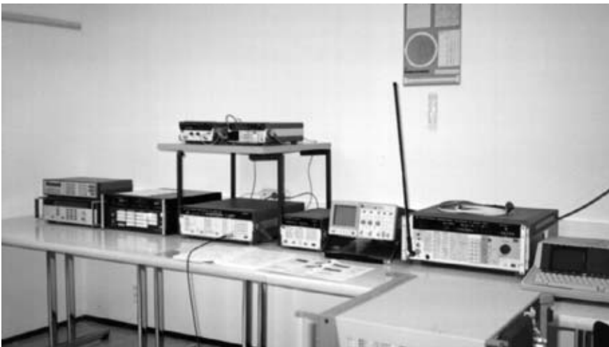
Figure 7.22 Essential calibration test instruments needed to keep the flying installation within its specifications.
