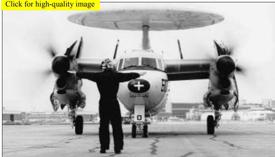
Hawkeye's 24-foot diameter rotodome houses a monopulse connected linear array of UHF yaggi antennas, and rotates at 5 rpm.
