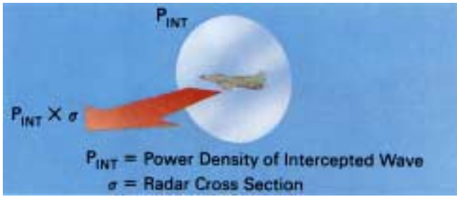
16. Density of power reflected in radar's direction equals density of intercepted wave times radar cross section.
