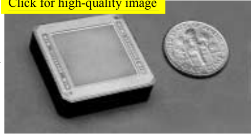
15. Dime-sized four-channel, three-dimensional T/R module.
