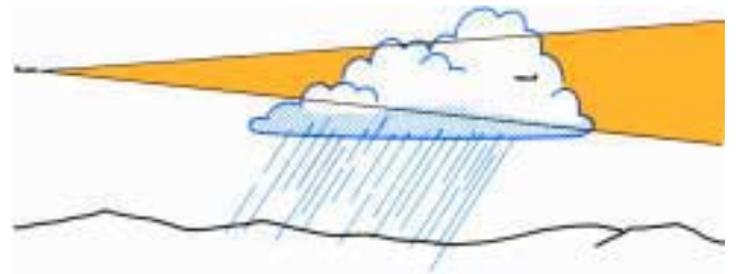
5. One of the many important losses not accounted for by the simple range equation is atmospheric attenuation.
