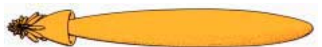
1. Three-dimensional plot of the strength of the radiation from a pencil beam antenna.
