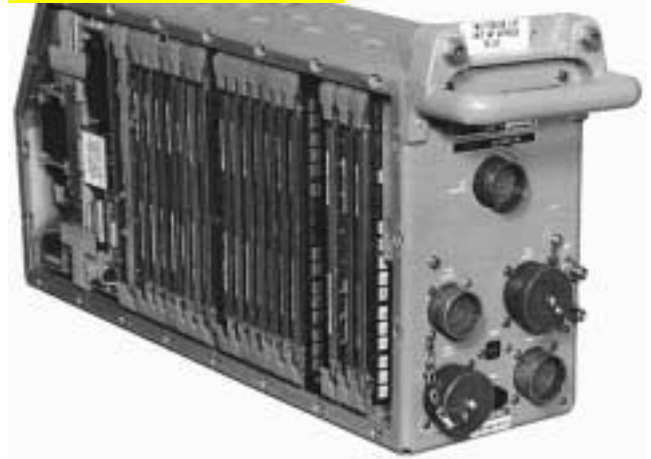
24. Signal processor. Stored program for the selected mode of operation is automatically entered by the data processor.
