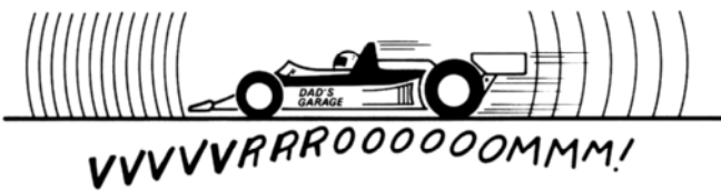
25. A common example of the doppler shift. Motion of car crowds sound waves propagated ahead, spreads waves propagated behind.
