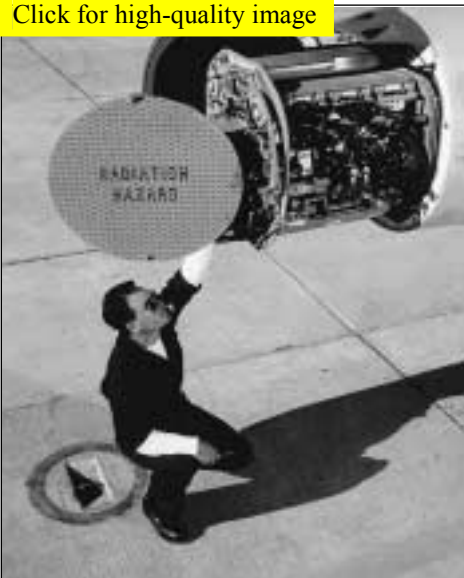
Radar, in F/A-18, consists of five easily accessible LRUs, all having front panel connectors.
