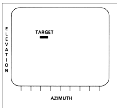
“C” Display. Shows target position on plot of elevation angle versus azimuth. Useful in pursuit attacks since display corresponds to pilot's view through windshield. Commonly projected on windshield as Head-Up Display.
