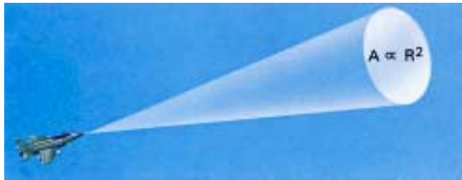
15. As waves travel out to a target, their power is spread over an increasingly large area.
