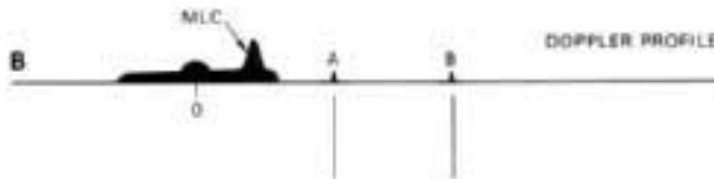
b) Doppler profile, without FM ranging—no clutter spreading.
