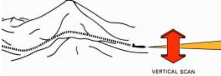
8. For terrain following, a radar scans the terrain ahead vertically with a pencil beam.
