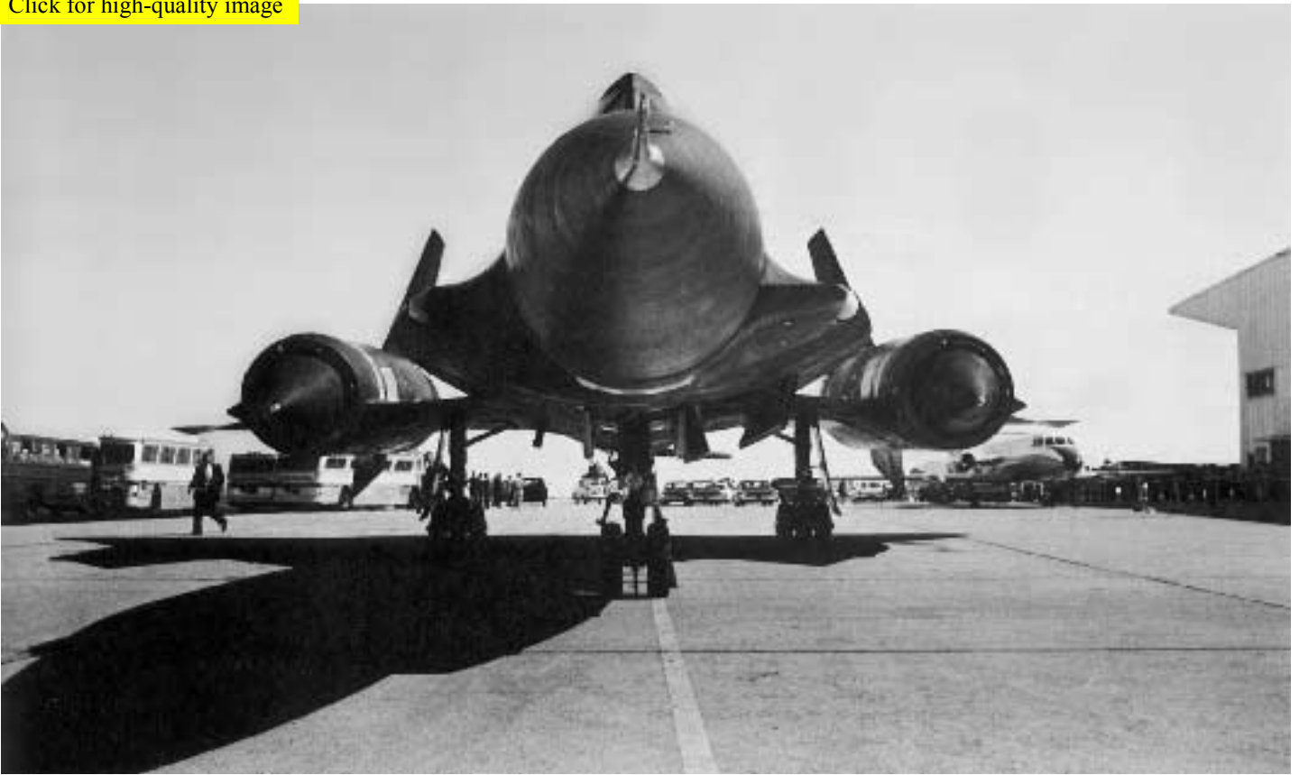
22. YF-12A of the early 1960s. First airplane capable of sustained Mach-3 flight; first interceptor to be equipped with a high PRF pulse-doppler radar.
