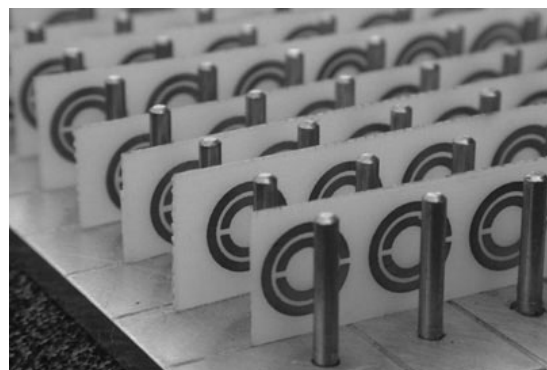
Figure 1.28 A left-handed material made from wires and rings. This picture is obtained from the homepage for Dr David R. Smith ( http://physics.ucsd.edu/~drs/index.html )
