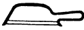
Hacksaw, sometimes appropriate for semi-rigid cable, although for repetitive operations a power trimmer should be considered
