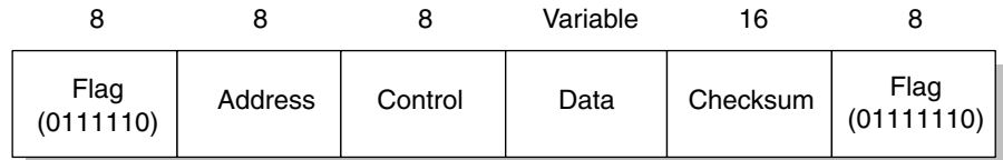
Figure 1-3 HDLC frame format.
