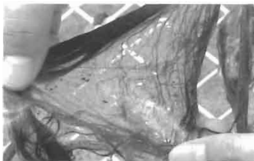
Fig. 2. Adhesive material spread to the membrane on carbon fiber surface.
