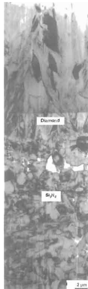
Fig. 14. Cross-sectional TEM micrograph of microstructure near an interface between diamond and \text{Si}_3\text{N}_4 .
