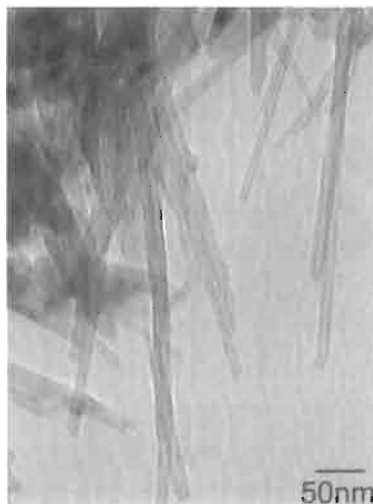
Fig. 14. TEM photograph of carbon nanotubes prepared from three-layered core/shell particles (PMMA/PAN/PMMA).
