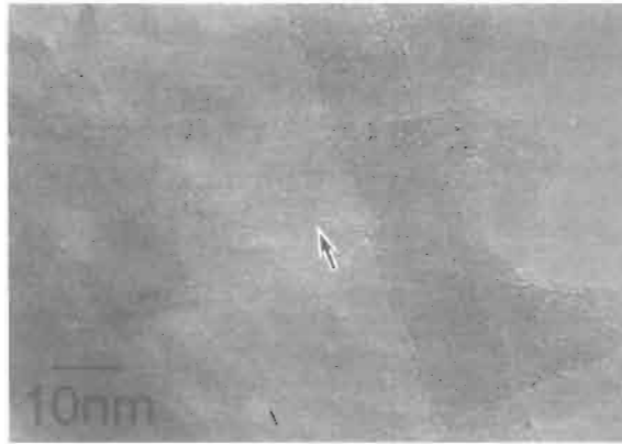
Fig. 12. TEM photograph of carbon nanotubes prepared from core(PMMA)/shell(PAN) particles.
