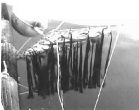
Fig. 1. Carbon fiber bundles attached to the experimental apparatus.
