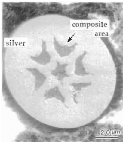
Fig. 7. Cross-sectional view of the drawn composite wire [10].
