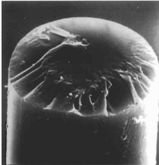
Fig. 2. Nicalon NL 200 room temperature fracture morphology.
