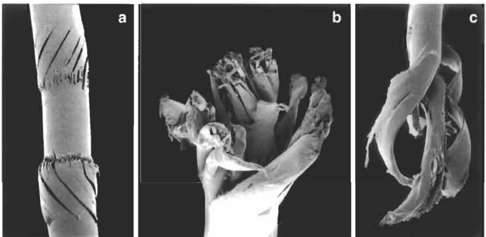
Fig. 11. Biaxial rotation fatigue. (a,b) Thick polyester fibre. (c) Finer polyester fibre. For further explanation, see Fig. 1.
