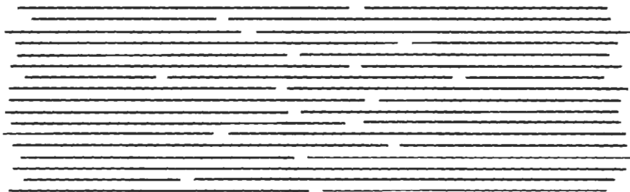
Fig. 4. Staudinger's (1933) view of the continuous structure of an oriented polymer.
