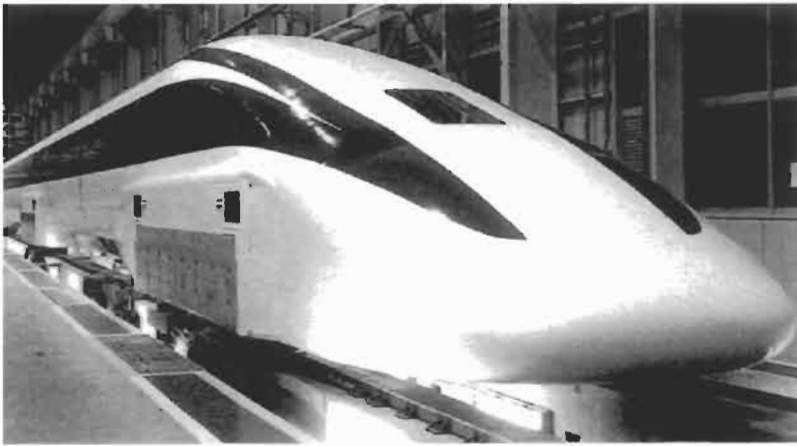
Fig. 15. Tested super-express linear motor cars (over 500 km/h). (Courtesy of Japan Railway Technical Research Institute.)
