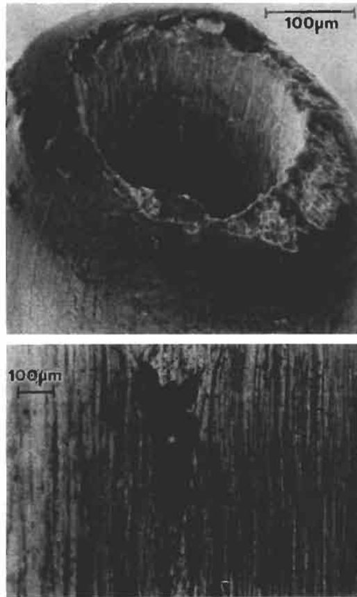
Fig. 3. Deep cup failure in a 0.45 mm diameter drawn Cu wire. The lower half shows a cup formed void (central burst). Reprinted from Murr and Flores (1998), Scripta Materialia , 39, p. 527, with permission from Elsevier Science.
