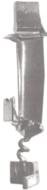
Figure 3.6 A single-crystal blade embodying a DS-starter block and helical constriction and a test plate facilitating orientation check by XRD.
