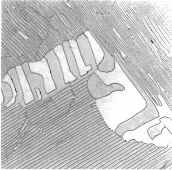
Fig. 51. Discontinuous coarsening of eutectoid in Co-Si alloys; a polycrystalline sample annealed at 1000°C for 96 h. \times 1875 . (From LIVINGSTON and CAHN [1974].)
