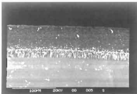
Fig. 36. Backscattered electron micrograph of a fully processed high activity pack aluminide coating on IN 738LC.
