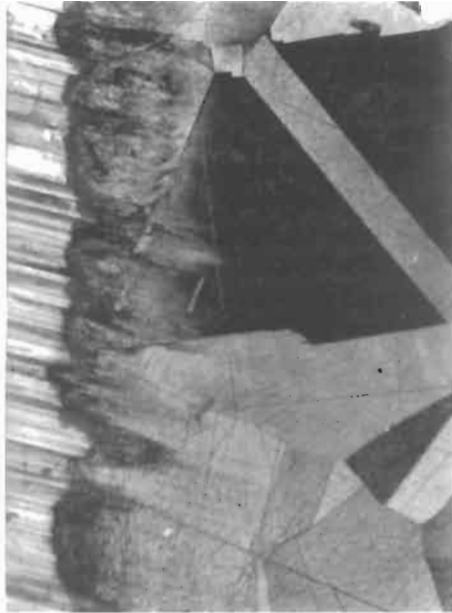
Fig. 2. Deformed layer in brass (CuZn 30) after cutting by a new diamond wheel. Oblique section ( 5^\circ to surface which is on the left side). Etched. 200 \times . (From KIESSLER et al. [1982].)
