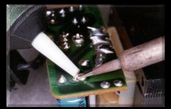
Ensure the pump is ready to go... (Left)The nozzle of the desoldering pump is applied to the molten solder and the springloaded plunger is then released, drawing the solder up into the pump. Repeat if needed.
