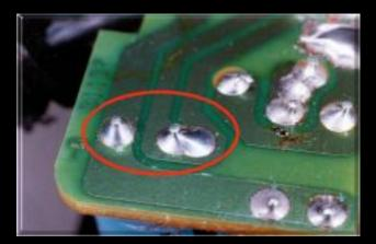
(Left) The two solder joints to be desoldered, to enable a faulty component to be removed.
