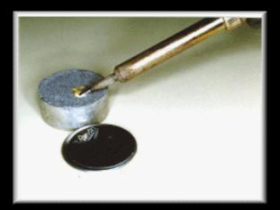
(Left) A useful product is Multicore's Tip Tinner Cleaner (TTC) - a 15 gramme tin of special paste which cleans and "tins" the iron, in one go. (Right) Insert components and splay the leads so that the part is held in place.
