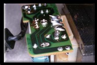
(**Right**) If using a <u>desoldering</u> pump, apply the iron first to melt the solder (1-2 seconds). Ensure the pump is 'primed' and ready to go...
