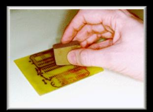
(Left) Boards must be clean to begin with, especially if they're not previously "tinned" with solder. Clean the copper tracks using e.g. an abrasive rubber block. (Right) Clean the iron "bit" (tip) using a damp sponge. Iron featured is an Ungar Concept 2100 Soldering Station.
