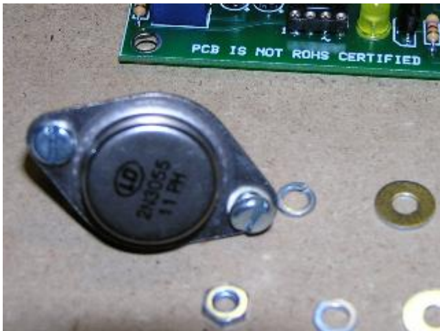
33. Next insert the two screws into the 3055 Transistor.
