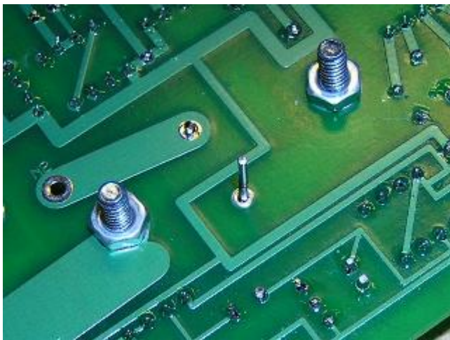
34. Insert the Transistor into place using the screws and leads to align it as straight as possible. And as with the diodes, cut ONE lead. Tighten the screw to help hold this in to position while you are soldering.
