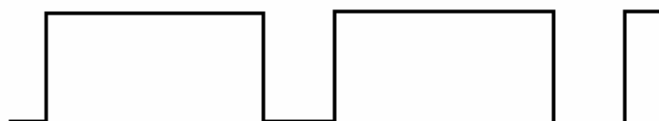
Square Wave - ON:OFF Ratio 3:1 Figure 4
