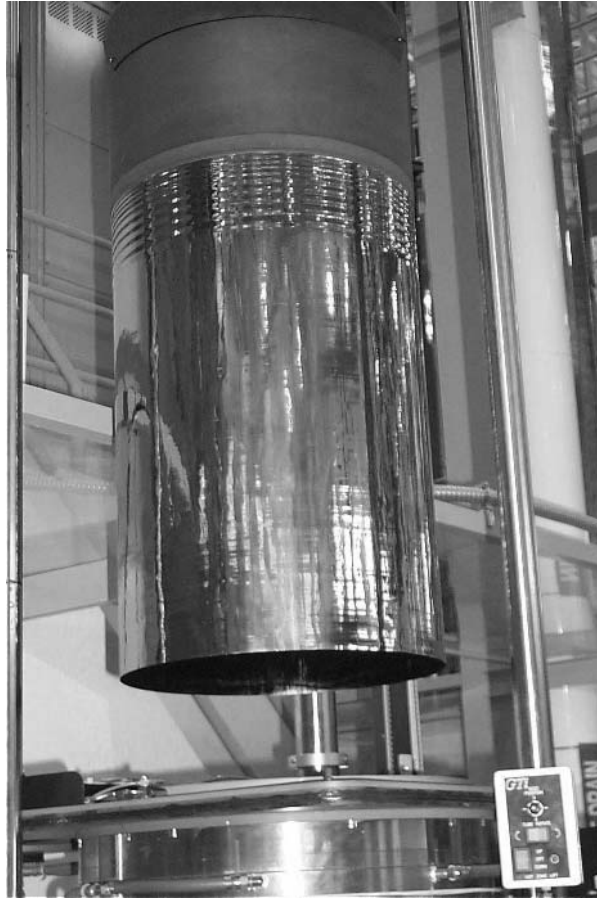
Figure 6.23 Experimental 50-cm-diameter EFG cylinder exiting from furnace
