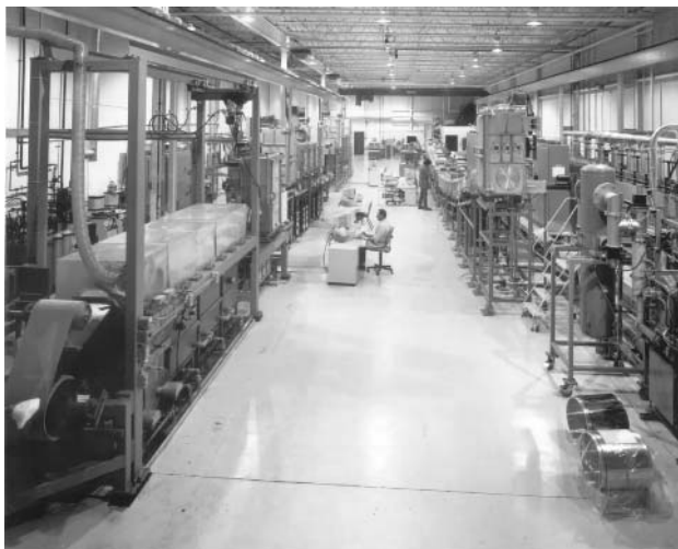
Figure 12.27 A photograph of the Energy Conversion Devices, Inc. 2-MW plant showing all four front-end roll-to-roll machines for washing, back reflector sputter deposition, PECVD deposition (right-hand side) and TCO deposition [185]
