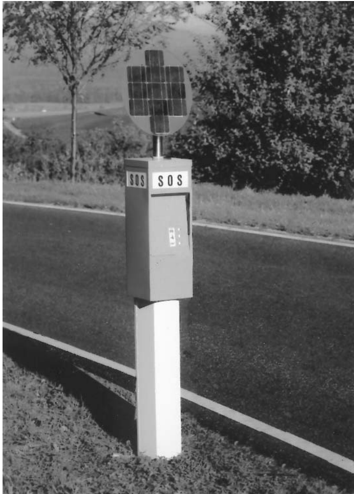
Figure 17.4 Photovoltaically powered emergency telephone (Source: Fraunhofer ISE, Freiburg)
