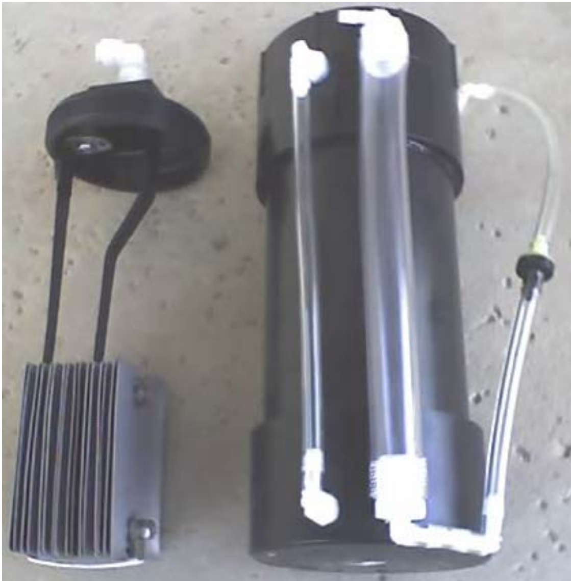
The picture above shows clearly the wall plates being used and how the bubbler is attached to the body of the booster with super-glue. It also shows the various pipe connections. The stainless steel switch-cover
