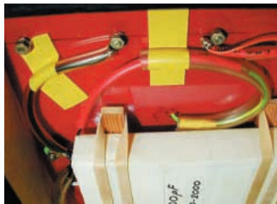
Using wooden strips and elastic bands to suspend the high voltage capacitor on the underside of the Pulser Unit.
