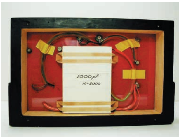
The high voltage capacitor mounted beneath the Tesla Transformer Unit.
