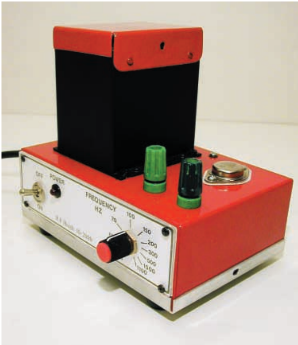
The completed Power Supply and Pulsing Unit showing the "shroud" protecting the mains transformer.
