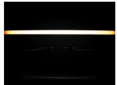
A fluorescent tube held close to the Tesla Transformer.
