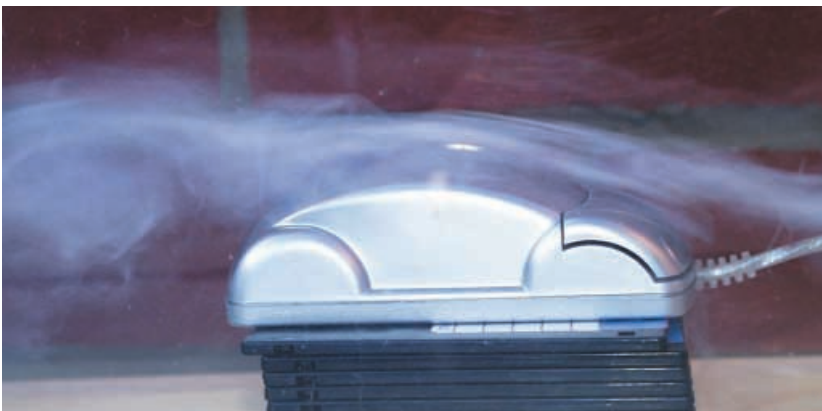
Smoke trail across a car-shaped computer mouse, using a plumber's smoke capsule as the source. Thinner trails from a nozzle-shaped source would provide better detail. Note how the air flows over the profile and then pulls back in towards the shape to fill the partial vacuum created.
