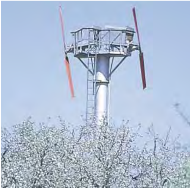
FIGURE 3.6 Wind machines mix cooler surface air with warmer air above.
