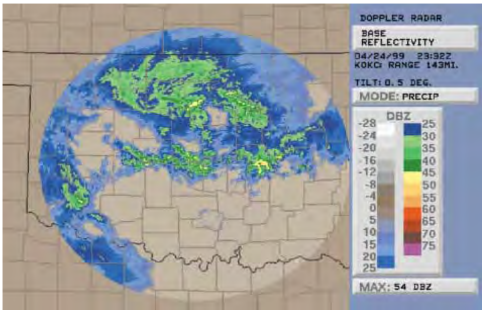
FIGURE 5.34 (a) Doppler radar display showing precipitation intensity over Oklahoma for April 24, 1999. (b) Doppler radar display showing 1-hour rainfall amounts over Oklahoma for April 24, 1999.
