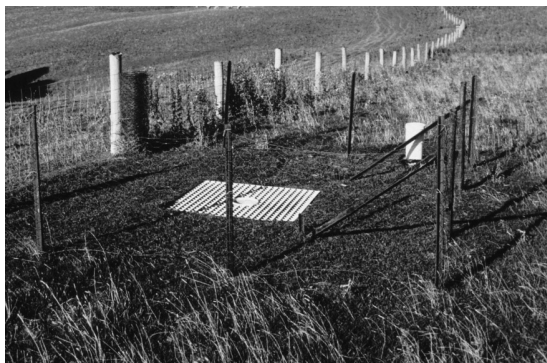
Figure 2.6 Surface rain gauge with non-splash surround.
