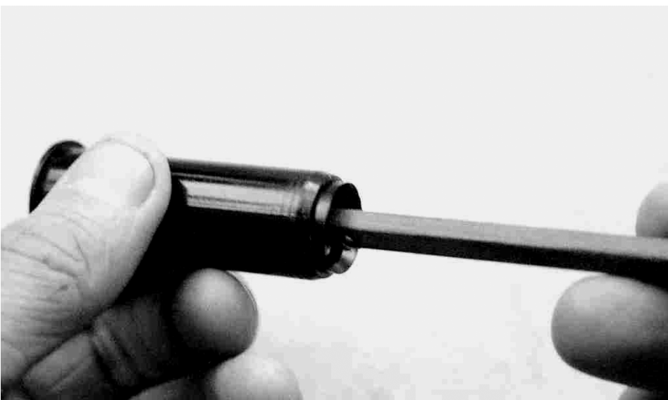
Press the cap home using a pencil.
