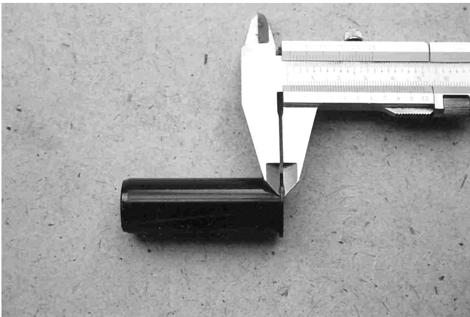
Checking the rim thickness. It should be 1- 1.5mm
