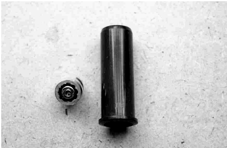
Primer assembly ready to fit to the case.
