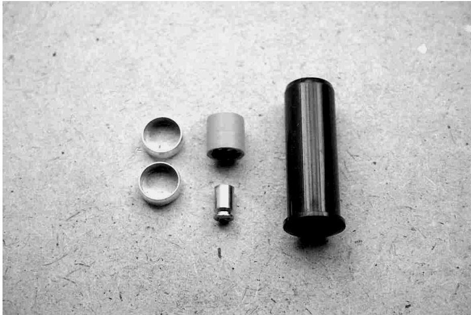
Gas tube and 8mm blank assembly.
