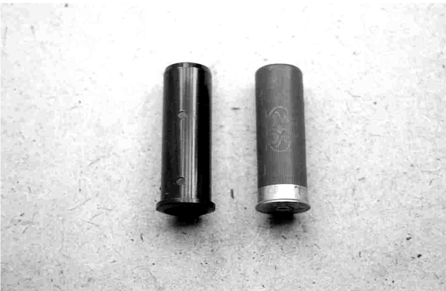
A 25mm pipe stiffener shown alongside a standard 12g shell.
