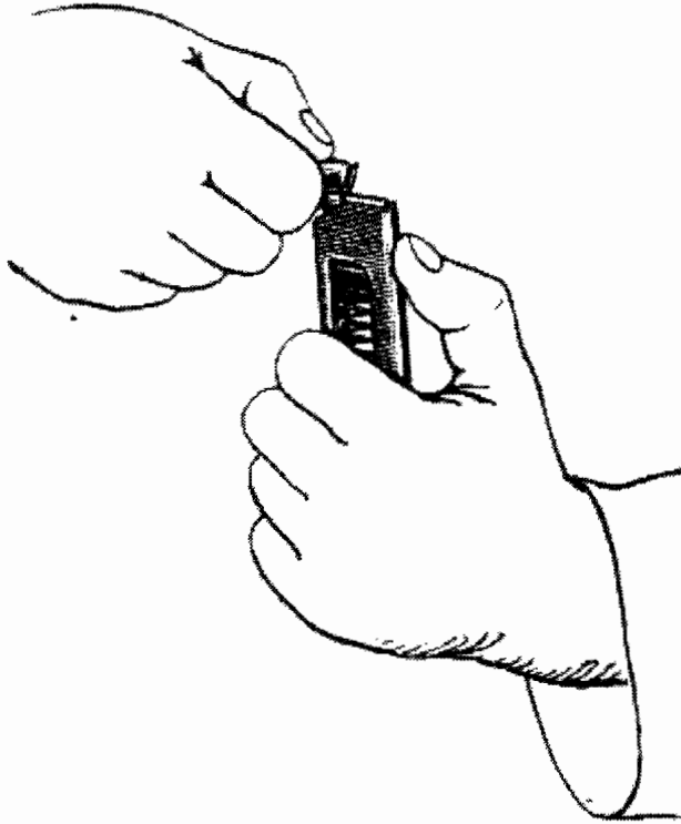
Picture 9.1 Loading the Magazine
