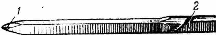
Picture 2.4 Firing Pin
