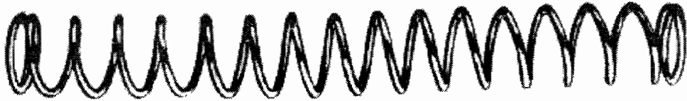
Picture 2.7 Recoil Spring
