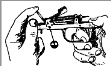
Figure 10: Releasing the hammer from cock
