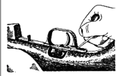
Figure 8: Depressing the trigger mechanism latch to remove the trigger mechanism
