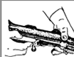
Figure 4: Removing the bolt assembly from the receiver
