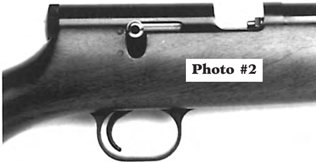
Photo #2 Striker handle in the "Fire" position. Striker handle is raised out of the safety notch. The striker handle will now be in line with the red dot on the stock. The rifle is ready to fire
