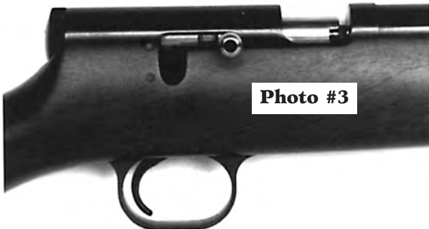
Photo #3 The Striker handle in the "Fired" Position. The striker is fully forward in contact with the nipple.
