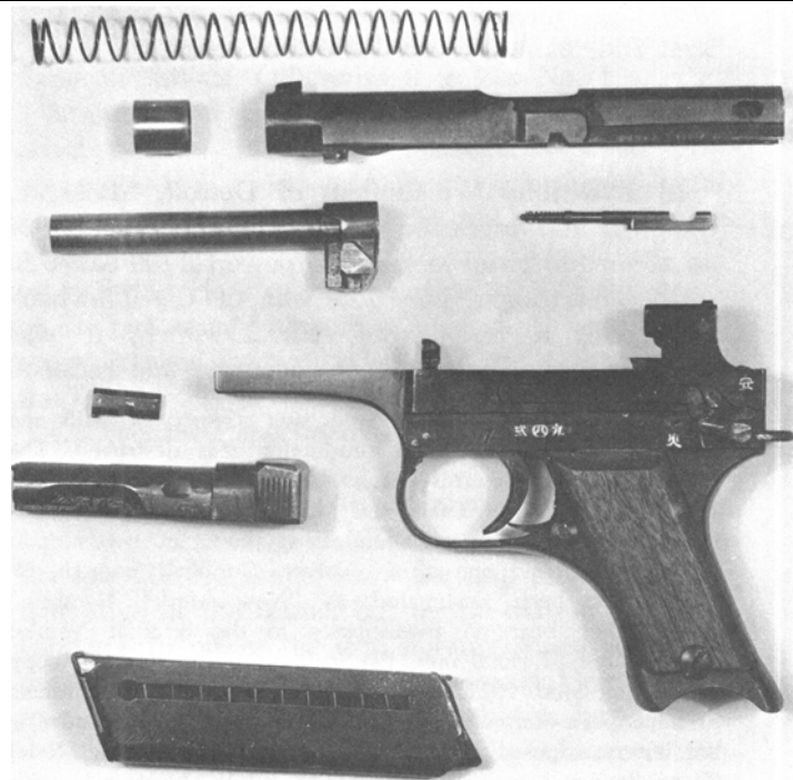
Fig. 177. 8 mm. Nambu Type 94 (1934). (Disassembled. Marked as made at the Nagoya Arsenal).
