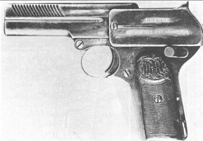
Fig. 149. 7.65 mm. Dreyse Mod. 1907. Specimen has variant serrations on finger grips.
