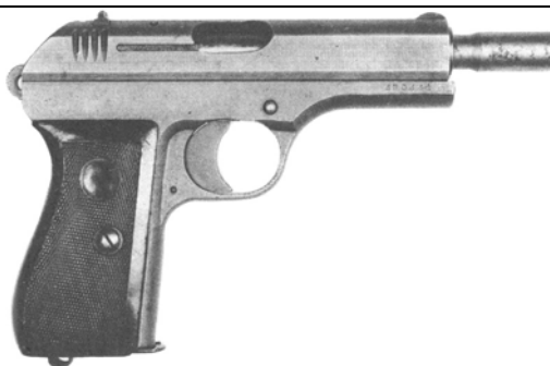
Fig. 143. 7.65 mm. Czech Mod. 27. Provided with silencer.
