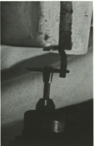
After measuring length of stem in relation to disconnector contact surface on secondary sear, trim stem to proper length.
