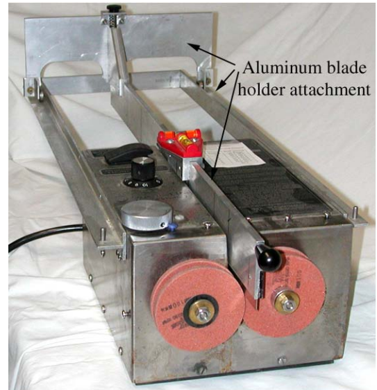
Figure A10 The TruHone sharpening machine with special attachment for grinding thin blades.
