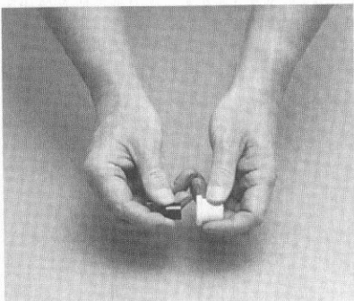
Epoxy thread protector into 3/4" x 1/2" bushing.
