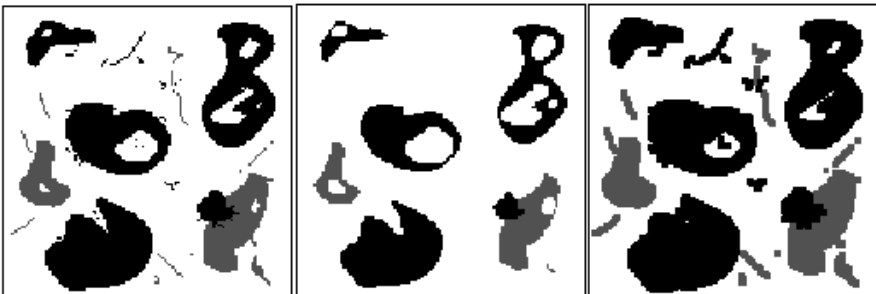
Figure 6.31 – Effects of erosion and dilation: original, eroded and dilated images from left to right respectively
