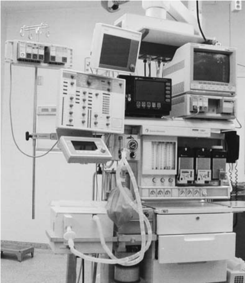
FIGURE 6 A full-service ventilator (such as the Servo 300A shown here) attached to the anesthesia machine can provide the same ventilator settings as used in the ICU, including pressure support and continuous positive airway pressure without the need to bring additional cumbersome equipment into the operating room.
