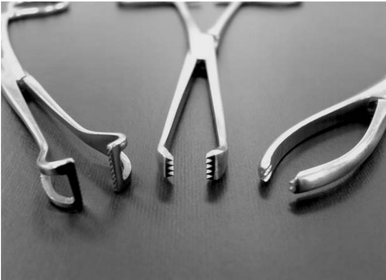
Figure 10.10 Close-up of the gripping surfaces of common ratcheted tissue forceps. From left: Babcock's, Allis, Littlewood's.
