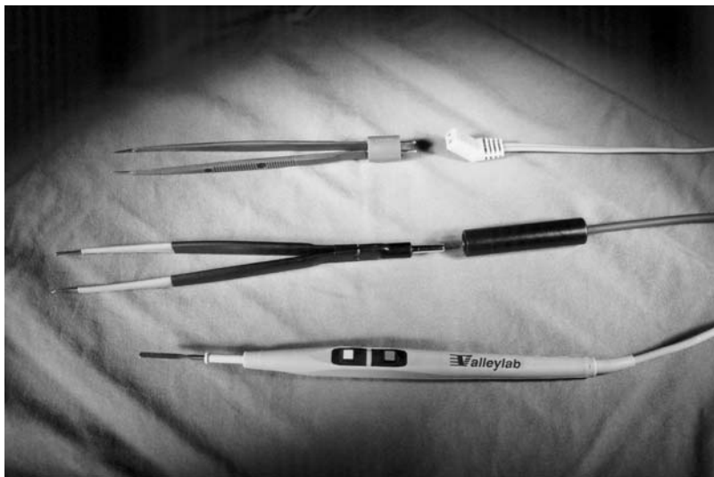
Figure 10.19 Common diathermy instruments. From top: bipolar diathermy forceps, monopolar diathermy forceps, monopolar blade diathermy. The forceps have not been plugged into their leads, to show that the bipolar forceps has two electrodes, while the monopolar has only one. Note the two control buttons on the blade diathermy: one is for cutting and the other for coagulation.
